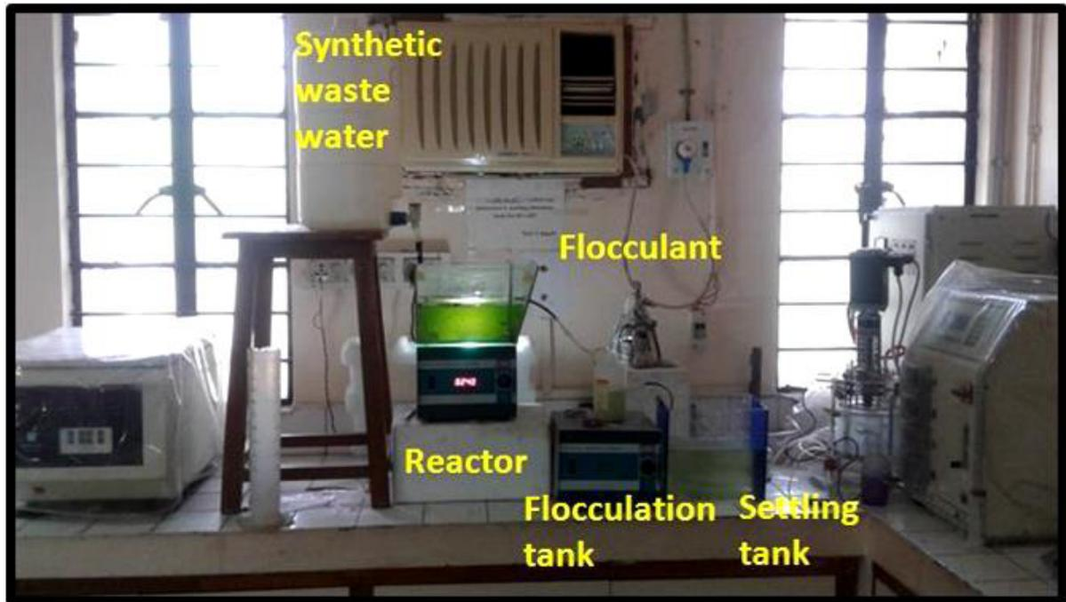
**Figure 3. 31** Continous reactor for the nutrient removal from wastewater.
