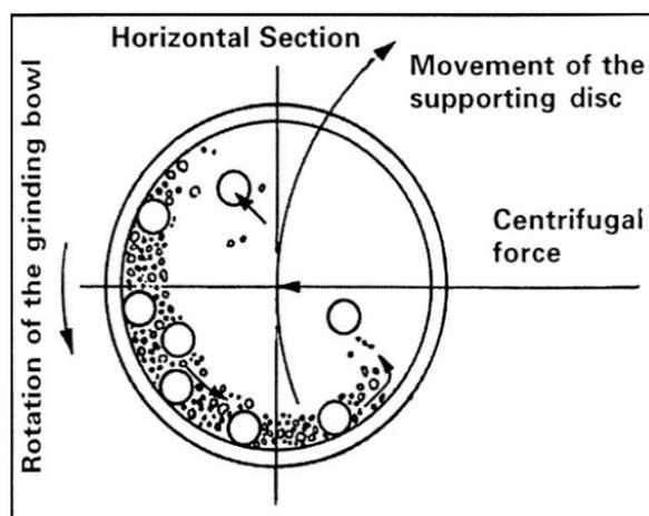
Fig. 3.2 The ball motion inside the milling jar and acting force on ball<sup>11</sup>.
