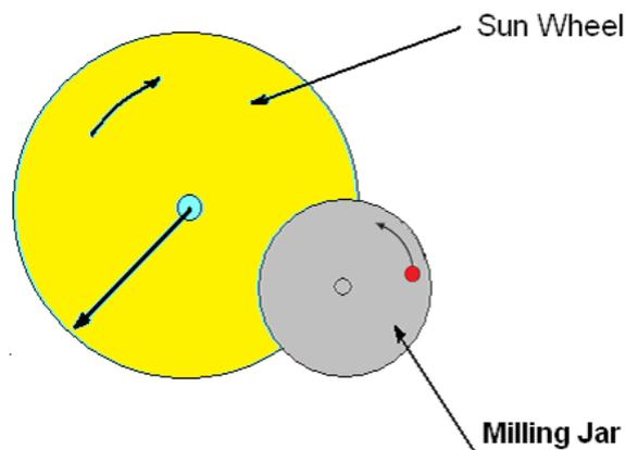
Fig 3.1 Arrangement of milling jar with sun wheel<sup>11</sup>.
