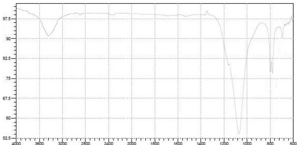
Fig.4.6 FTIR image of prepared nano-sized synthetic quartz sample.
