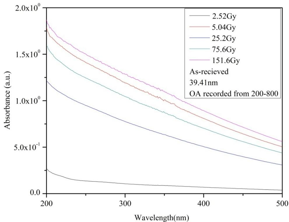
**Fig.4.7** UV-Visible spectra of prepared un-annealed nano-sized synthetic quartz sample.
