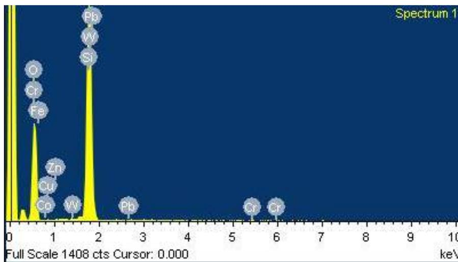
**Fig.4.5** EDX image of chemically treated nano synthetic quartz sample.
