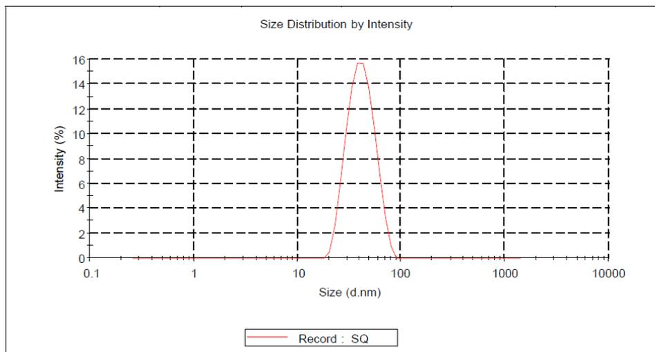
**Fig. 4.1** Representation of average particle size and PDI of un-annealed nano synthetic quartz sample
