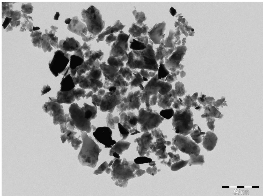
**Fig.4.3** TEM image of un-annealed nano synthetic quartz sample.
