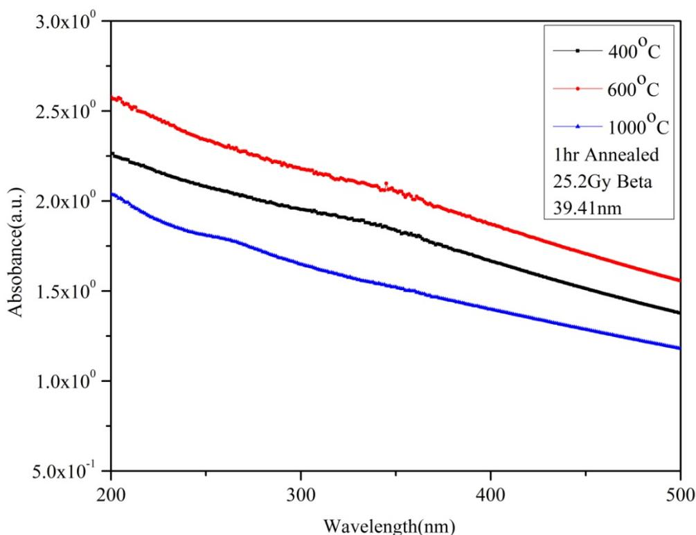
**Fig.4.8** UV-Visible spectra of prepared nano-sized synthetic quartz samples annealed at 400°C, 600°C and 1000°C.
