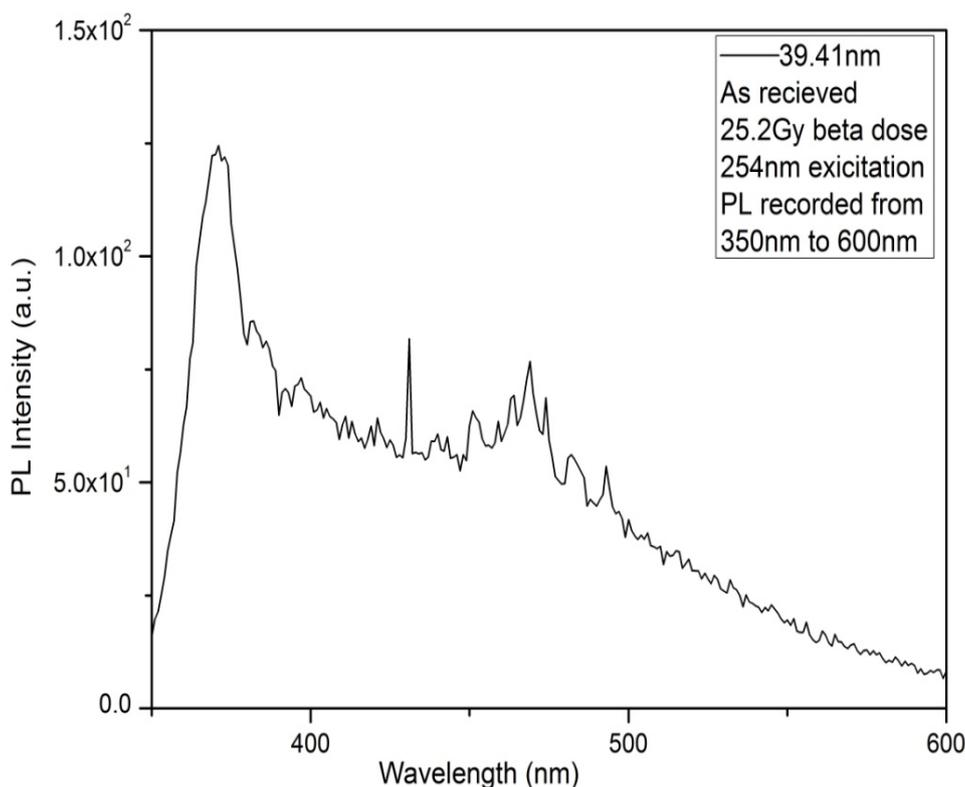
**Fig.4.9** PL emission spectra of un-annealed nano synthetic quartz sample.
