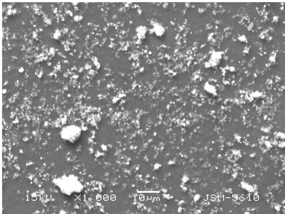
**Fig.4.2** SEM image of un-annealed nano synthetic quartz sample.
