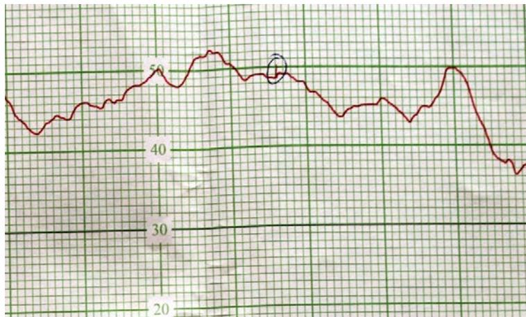
**Fig. 5.29** ESR spectra for 1000°C annealed NSQ sample irradiated with 55Gy.
