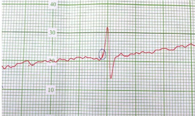
**Fig. 5.28** ESR spectra for 600°C annealed NSQ sample irradiated with 55Gy.
