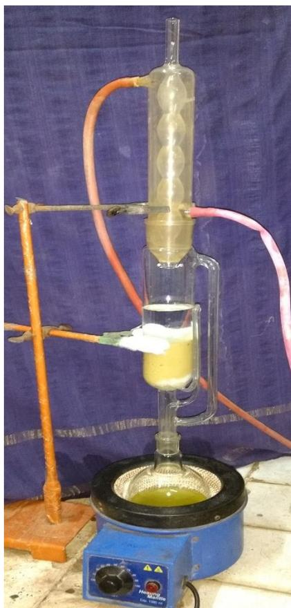
**Figure 2.2** Setup for Soxhlet extraction of non-polar phytocomponents of *Aloe vera* gel
