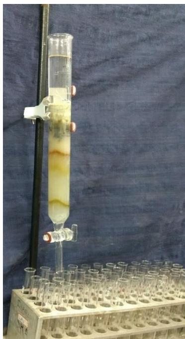
**Figure 2.3** Setup for column chromatography
