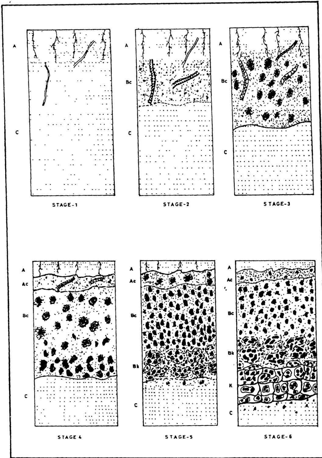
Fig.4.7 Stages of calcretization—Fine textured soils.
