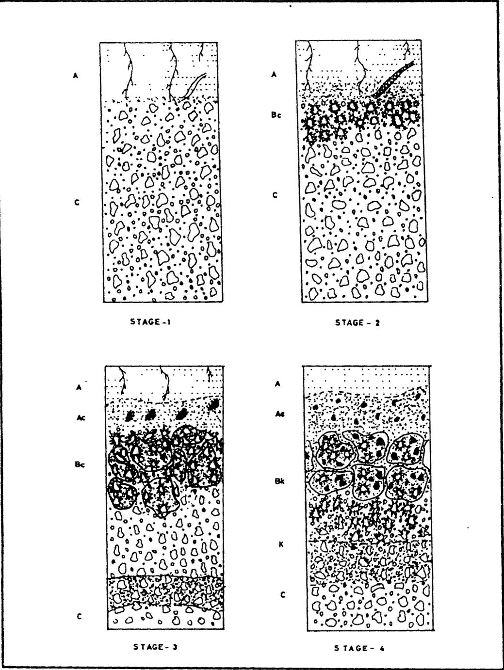
Fig. 4-8. Stages of calcretization - Coarse textured soils.
