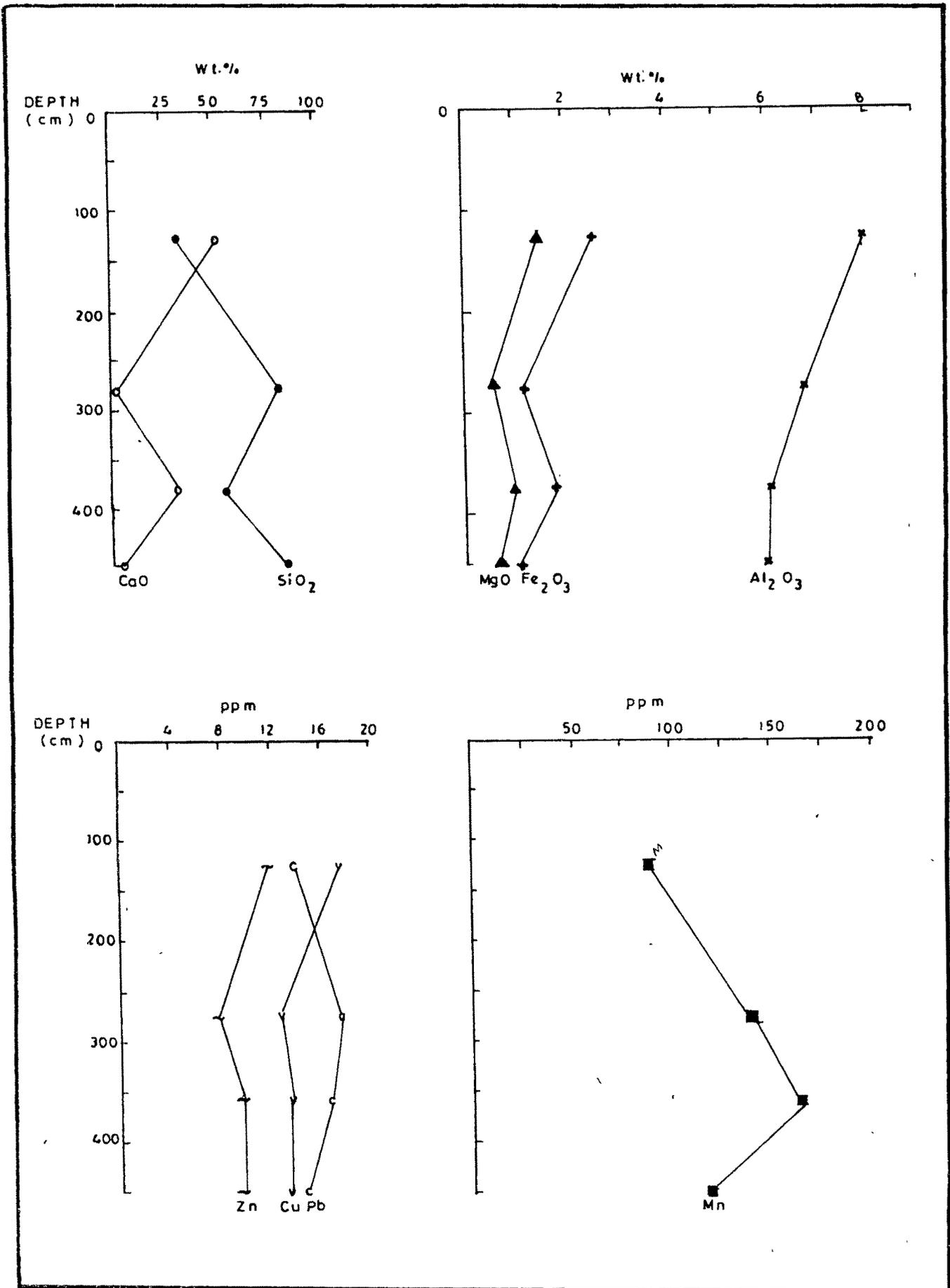
Fig.4-3-F. Major oxides, trace element chemistry – Belwa profile.
