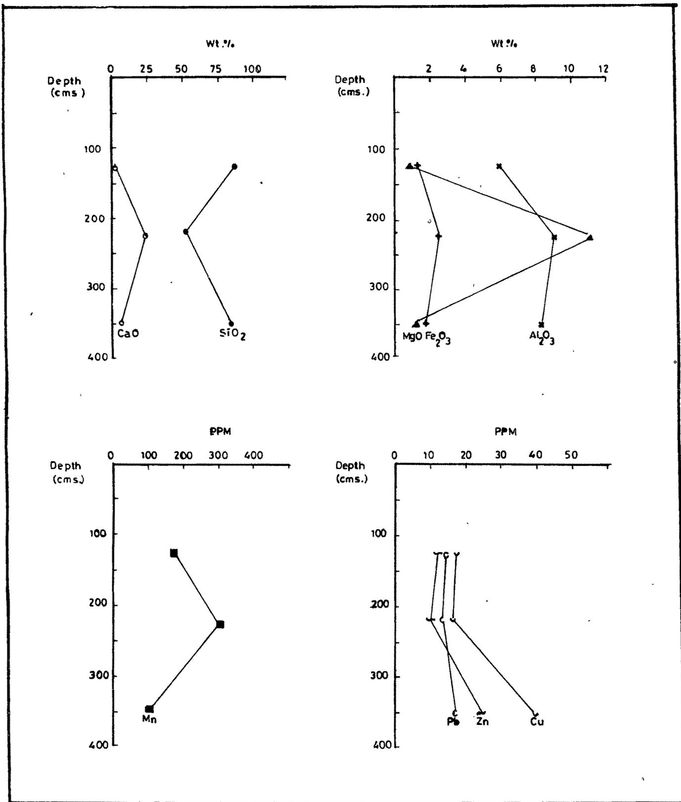
Fig. 4-3-E. Major oxide, trace element chemistry – Bhaleri profile.
