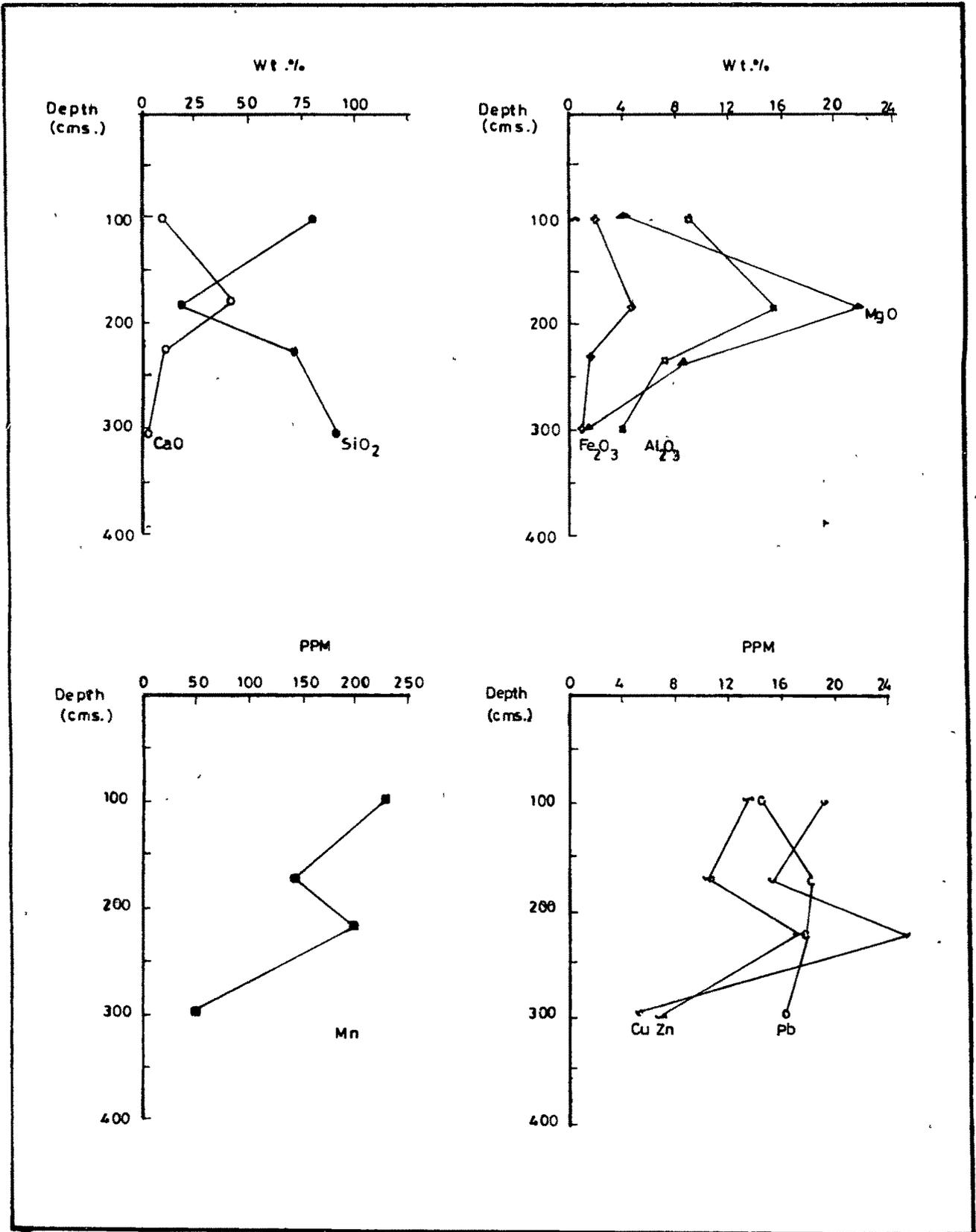
Fig. 4-3-D Major oxide, trace element chemistry – Sardarsahar profile.
