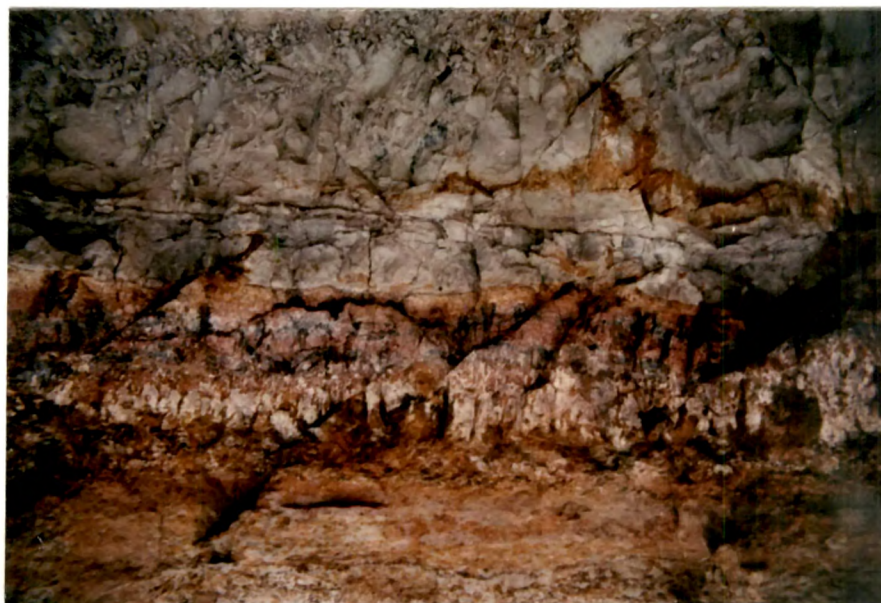
Plate-XI Mine section showing the various colour bands within the bentonite.
