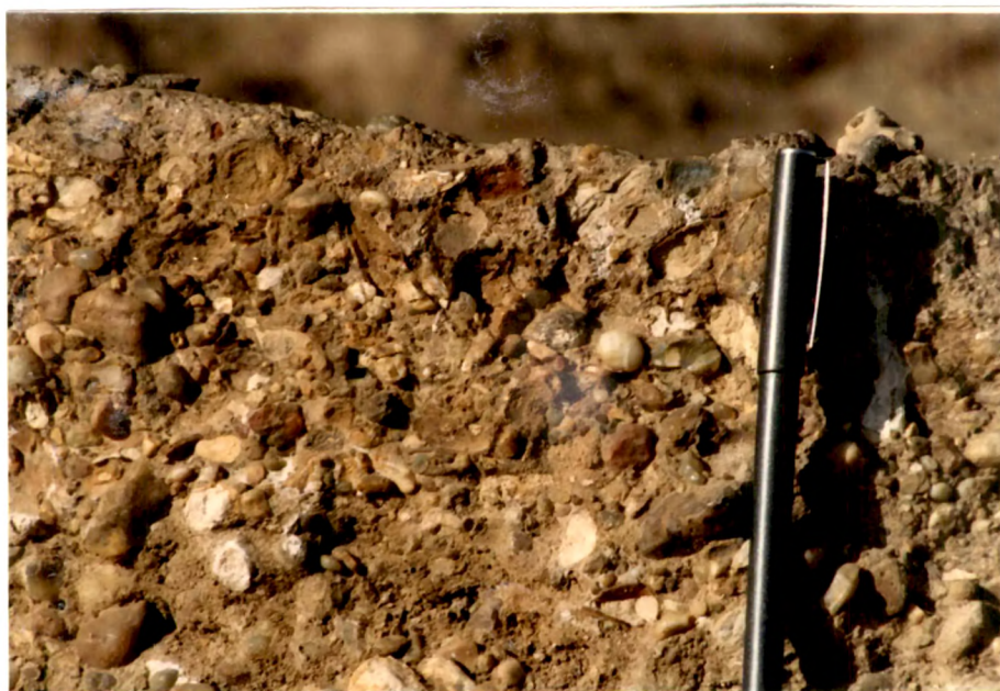
Plate-XX Rounded pebbles of agate and chalcedony cemented in a siliceous clay matrix.
