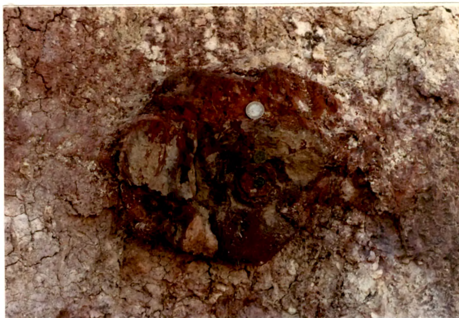
Plate-III Relicts of spheroidal weathering preserved within the bentonite.
