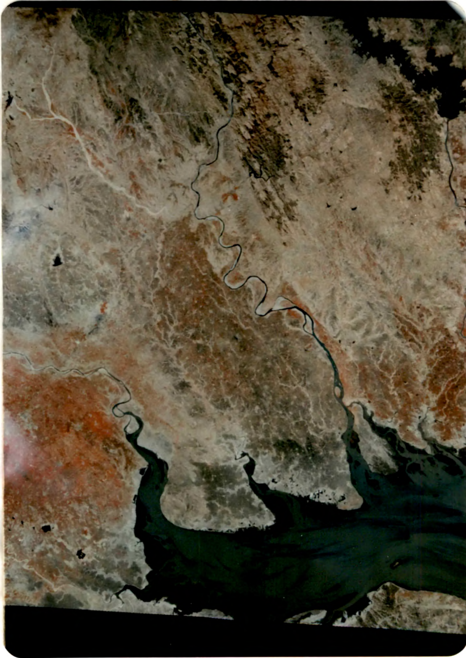
PLATE III.1 A view of the study area and adjoining region as seen in LANDSAT - 5 (TM band 2,3 and 4; Resolution 30m) showing geomorphic setup, features of structural controls and terrain characteristics
