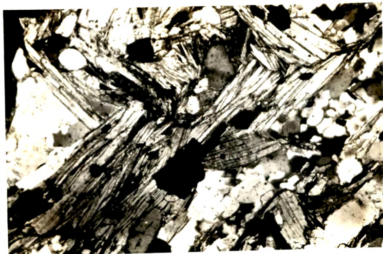
Mica schist showing the microfolding of an earlier foliation. (Photomicrograph: Cross nicols, X75)
