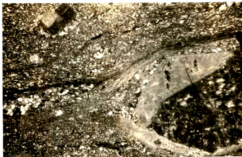
Sheared gneiss with a partly altered plagioclase porphyroblast embedded in a finely granulated matrix (Photomicrograph: Cross nicols, X30)
