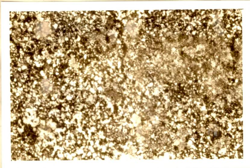
Cherty quartzite showing streaks and patches of calcite. (Photomicrograph: Cross nicols, X75)
