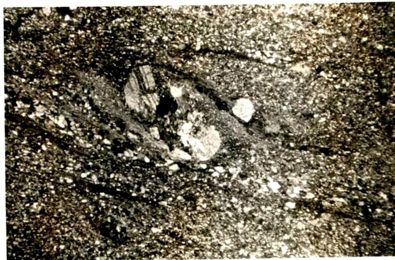
Siliceous tuff showing broken and deformed sodic plagioclase. (Photomicrograph: Cross nicols, X30)
