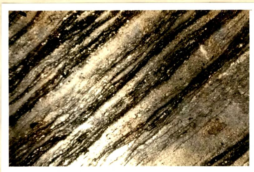
Slate consisting of light and dark coloured laminae. (Photomicrograph: Polarised light, X30).
