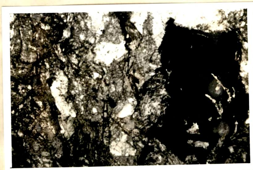
Diabase showing skeletal crystals of ilmenite with leucoxene. (Photomicrograph: Polarised light, X30)
