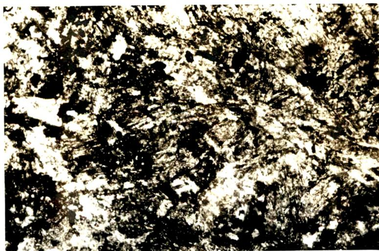
Texture of foliated diabase showing broken and altered feldspar embedded in chlorite and uralite. (Photomicrograph: Cross nicols, X75)
