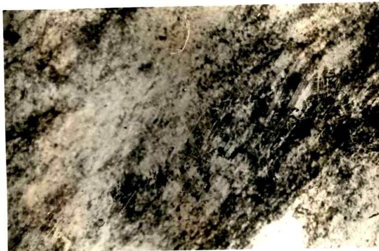
Siliceous tuff showing deformed patches of volcanic glass. (Photomicrograph: Polarised light, X30).
