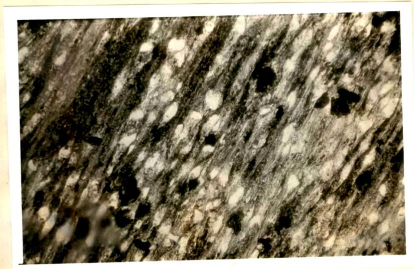
Tuffite showing a uniform scattering of quartz grains in a foliated volcanogenic matrix. (Photomicrograph: Polarised light, X30).
