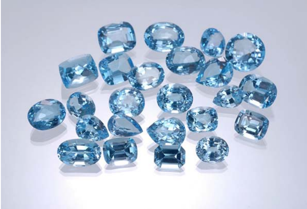
Fig. 5.2 Photograph showing Topaz treated by high energy electrons from a linear accelerator results in the Sky Blue colour.
