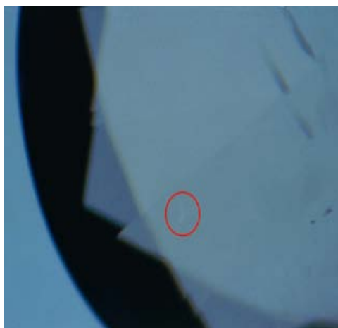
Fig. 6.4 Photograph showing exfoliation of coating in Methylene Iodide (under microscope 100X).
