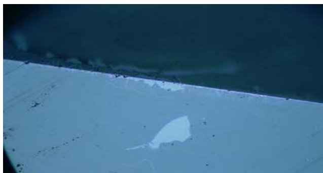
Fig. 6.5 Photograph showing exfoliation of coating under microscope.
