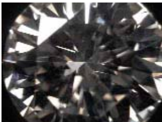
Fig. 7.2 B Photograph showing the flash effect is negligible in the gemstone which is treated by lesser drill method.
