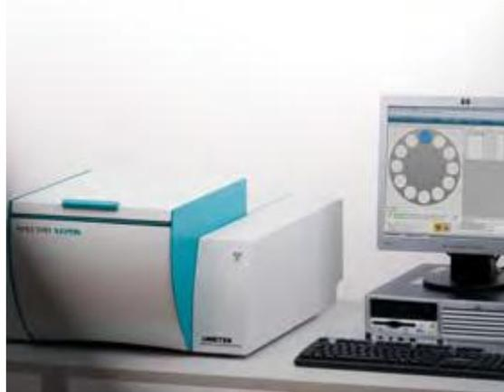
**Fig. 5.9** X-Ray Fluorescence Spectroscopy (XRF) machine Spectro Xepos He.
