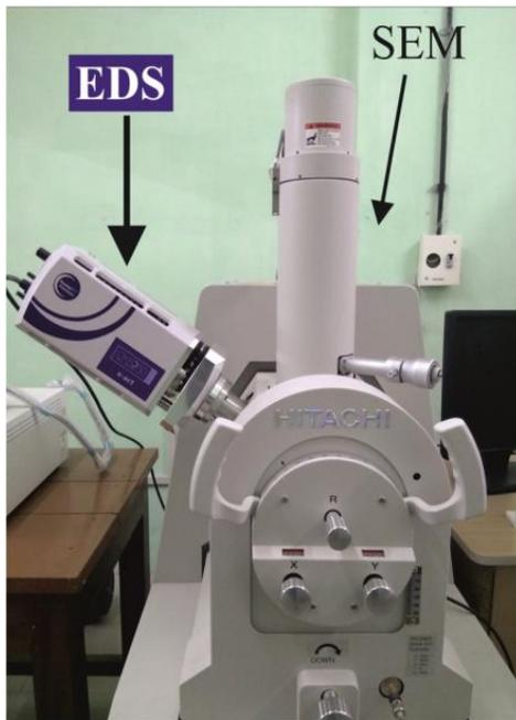
**Fig.5.5 a.** Scanning Electron Microscope (SEM) Hitachi, Germany.
