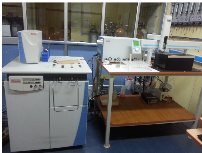
Figure 3.11: Photo shows Thermo Fisher Delta-V Plus IRMS on the left and Pal Gas-bench to the right at PRL.
