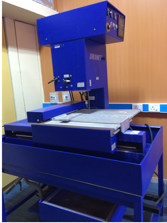
Figure 3.1: Dramet cutting machine at PRL used to slice speleothems.
