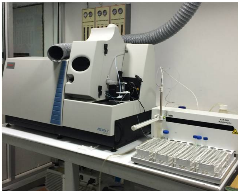
Figure 3.14: Thermo-scientific Quadrupole-Inductively Coupled Plasma mass spectrometer at PRL, Ahmedabad.
