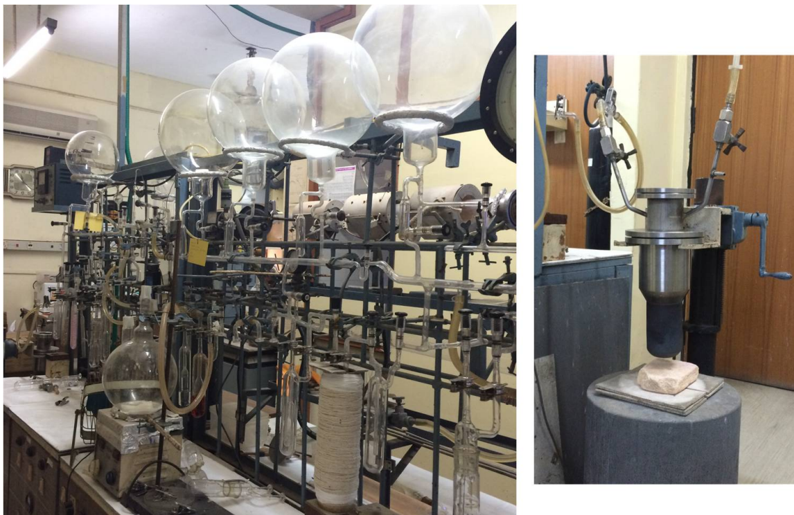
Figure 3.16: Photo shows the benzene synthesis glass line at PRL on the left and reaction chamber on the right.
