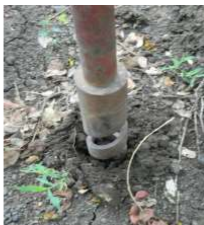
Plate 5. 1a Field Photo Depicting process of Augering for Soil Sampling
