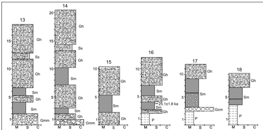
**Figure 6.5** Lithologs of bajada sediments exposed in the Nandikhadi River. Locations are shown in Fig. 6.1D. The vertical scale is in meters.
