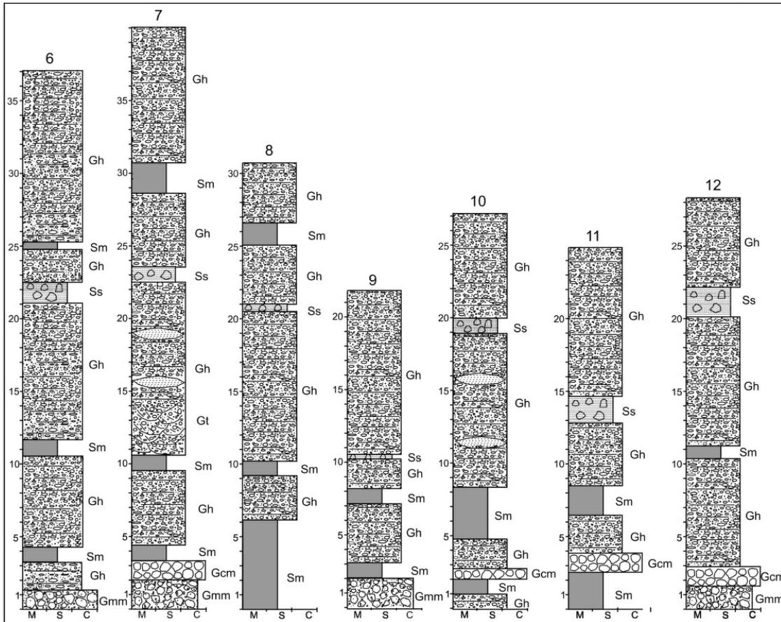
**Figure 6.4** Lithologs of bajada sediments exposed in the Nandikhadi River. Locations are shown in Fig. 6.1D. The vertical scale is in meters.
