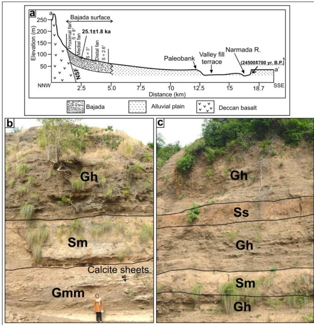
**Fig 6.2** (A) Topographic cross profile of the bajada surface drawn from the DEM. Note the wedge shaped coarse gravelly bajada sediments deposited in front of the mountain front. Three sectors of bajada surface and their slopes are also shown. (1- Allchin et al., 1978). (B) View of the cliff section exposing bajada sediments at site 10. Note the parallel horizontal calcite sheets formed in basal matrix supported gravel lithofacies. (C) View of the cliff section at site 11.
