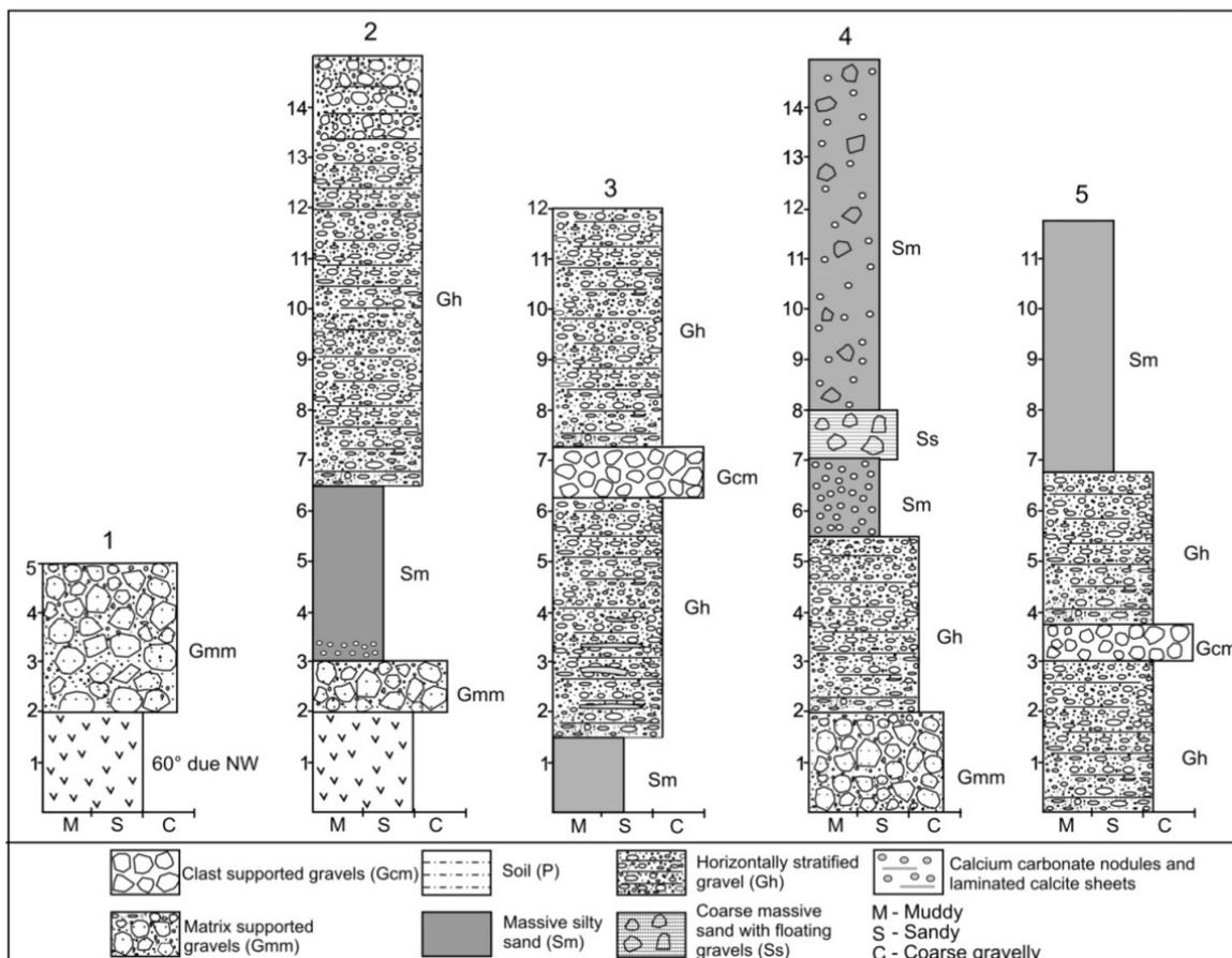
**Figure 6.3** Lithologies of bajada sediments exposed in northward flowing unnamed rivers located to the west of Nandikhadi River. Locations are shown in Fig. 6.1D. The vertical scale is in meters.
