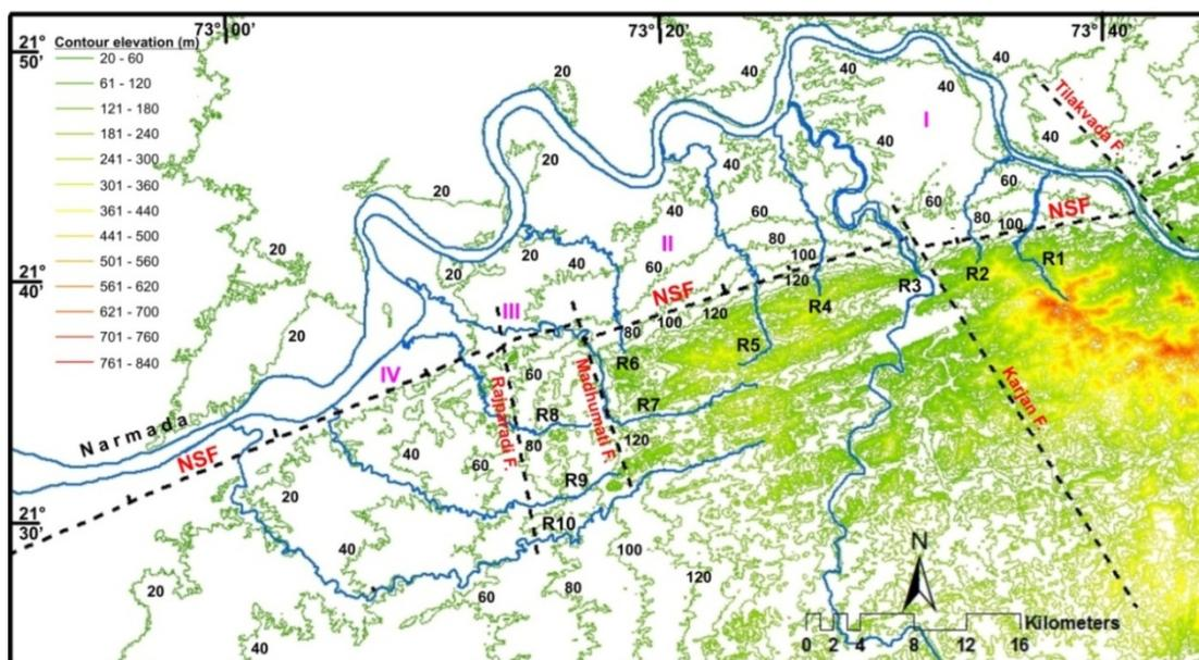
**Figure 4.4** Contour map of the study area with drainage and fault lines. Note the ENE–WSW trending north-facing scarps of the NSF and the gentle northward slope of the alluvial plain.
