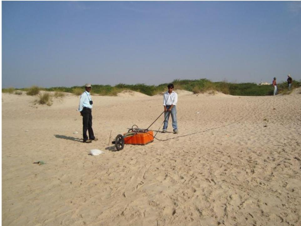
**Figure 4.7:** Field photograph showing GPR survey on Layza coast
