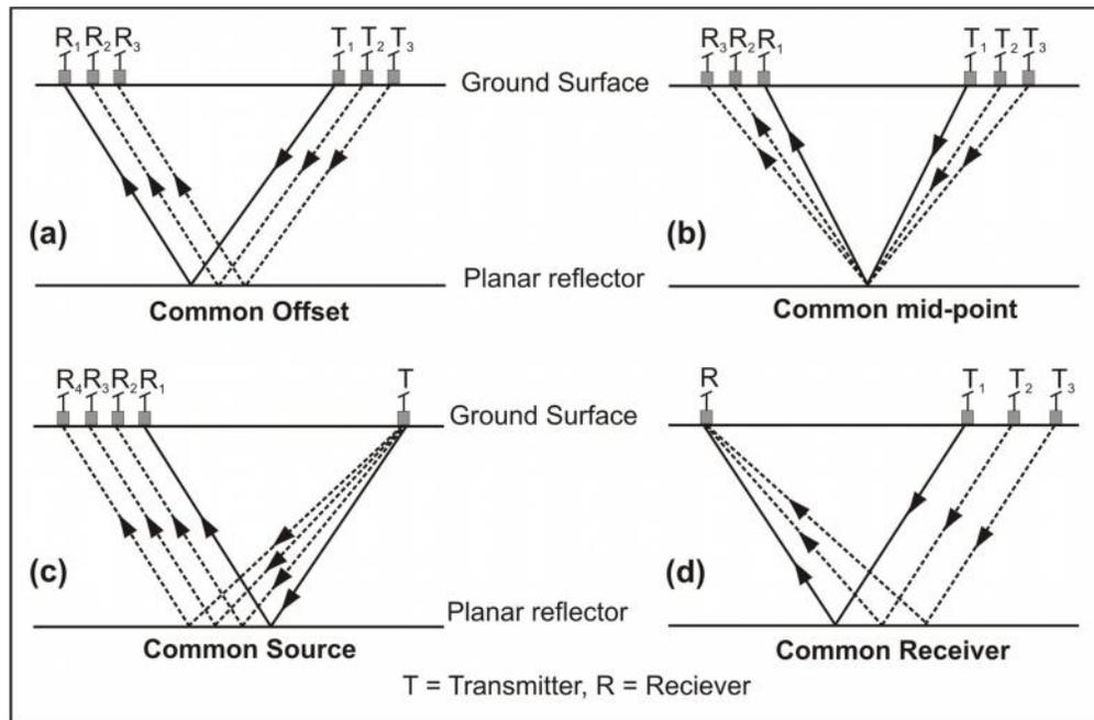
**Figure 4.4:** Modes of bistatic GPR survey (After Neal, 2004).
