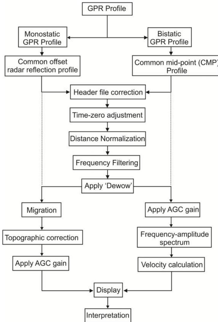
**Figure 4.5:** GPR data processing sequences for monostatic and bistatic antennas based on geophysical softwares developed by various commercial agencies. (Chamyal et al., 2007)
