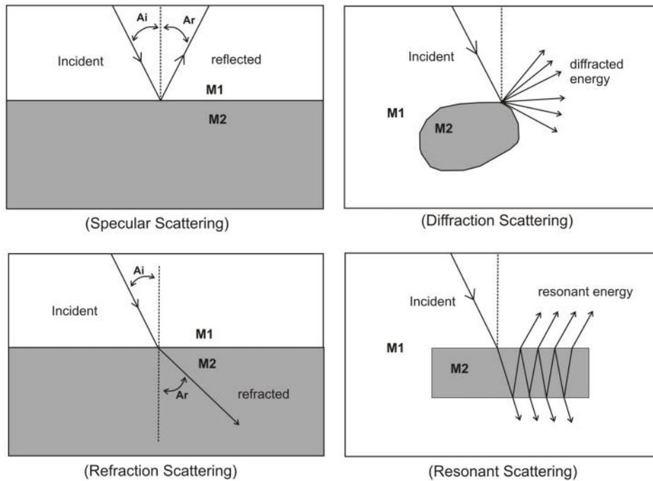
**Figure 4.2:** General scattering patterns for radar waves (a) specular reflection scattering (b) refraction scattering (c) diffraction scattering (d) resonant scattering (after Daniels, 2000).
