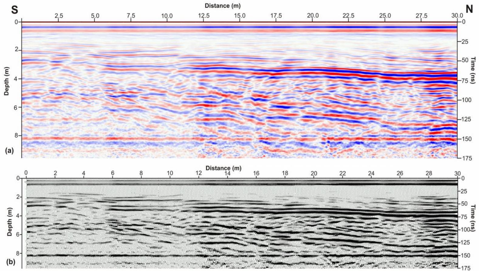
**Figure 4.9:** GPR profiles of Dhrabudi coast. (a) 200 MHz GPR Profile from the Dhrabudi temple coast shown in scan mode. (b) 200 MHz GPR Profile from the Dhrabudi temple coast shown in wiggle mode.
