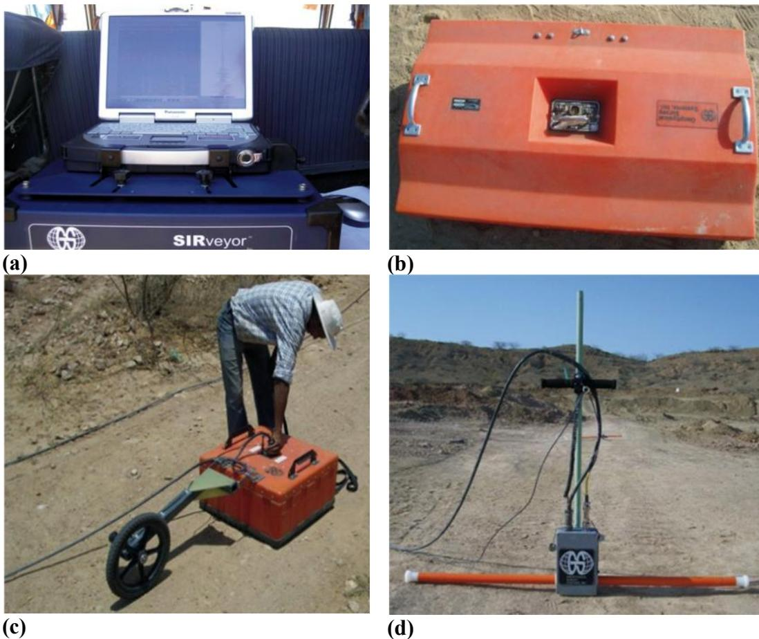
**Figure 4.3:** GSSI SIR-20 GPR with its different components. (a) Control unit mounted with toughbook system computer, (b) Shilded monostatic antenna of 100Mhz frequency, (c ) shilded monostatic antenna of 200Mhz attached with survey wheel and (d) bistatic unshielded receiver antenna of 80Mhz frequency which can be changed by extending the length of horizontal rods.
