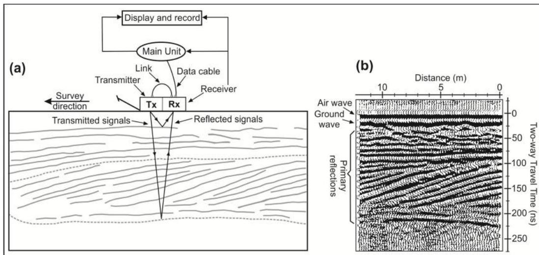
**Figure 4.1:** GPR data acquisition and the resulting radar profile in wiggle mode. (a) The GPR system components, manner of signal penetration and internal architecture of the subsurface reflectors. (b) GPR reflection profile in wiggle mode. Position of Ground waves, Air waves and primary reflections are indicated (after Neal, 2004).
