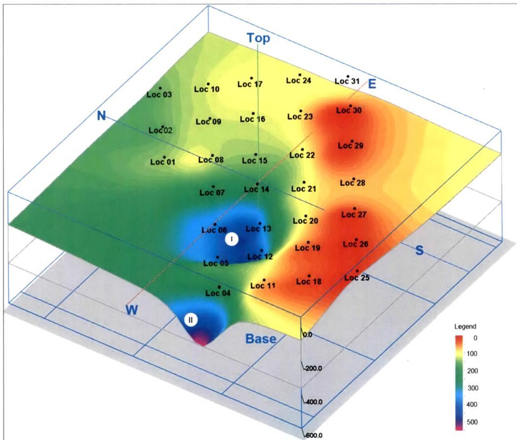
Figure 3-: Late Tertiary–Early Quaternary palaeo-topography of area under study in the lower reaches of Narmada valley. I and II are the depressions carved over Late Tertiary–Early Quaternary surface forming the sites of thickest Quaternary sediment in the study area.
