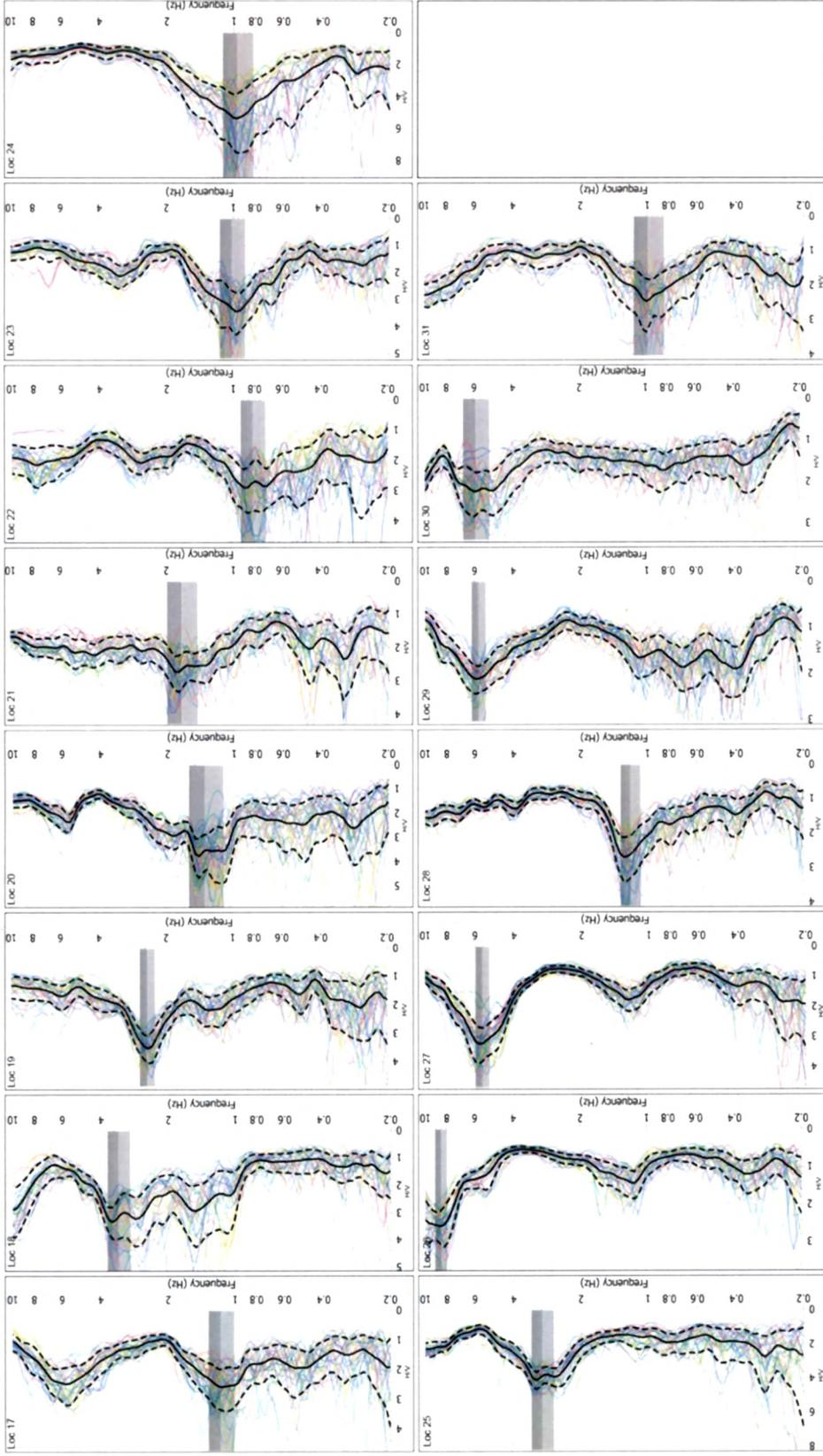
Figure 3:- H/V spectral ratio for 31 stations (frequency range 0.2–10 Hz). The coloured thin lines are H/V spectral ratio for different windows, black solid line is the average value and black dashed lines are  $\pm$ standard deviation. The bar shows the fundamental frequency with two grey shades representing  $\pm$ standard deviation.
