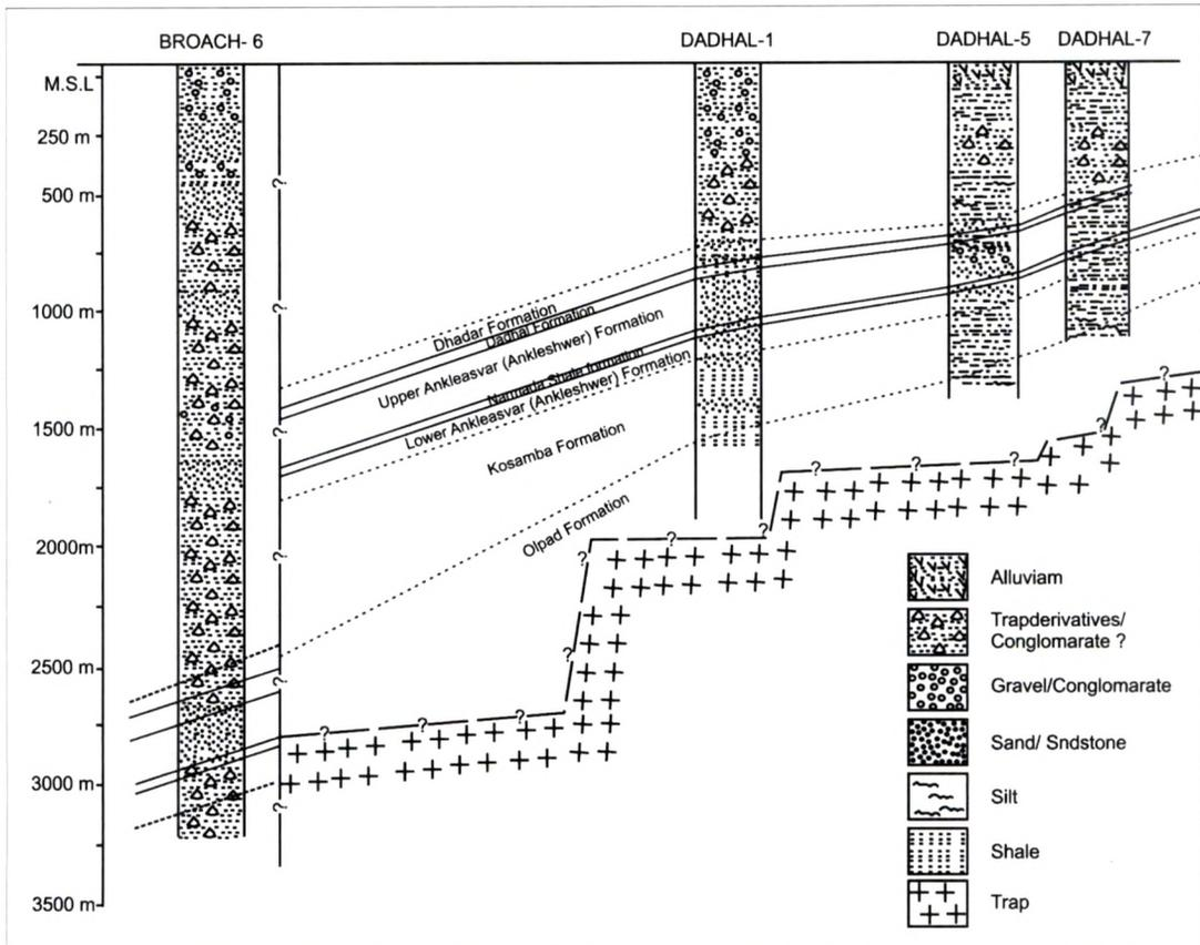
Figure 3:- Image showing borehole correlations from the available boreholes in the present study area (adopted from Rao (1969), Fig. 2, p. 27). See Figure 3-1 for location of boreholes.
