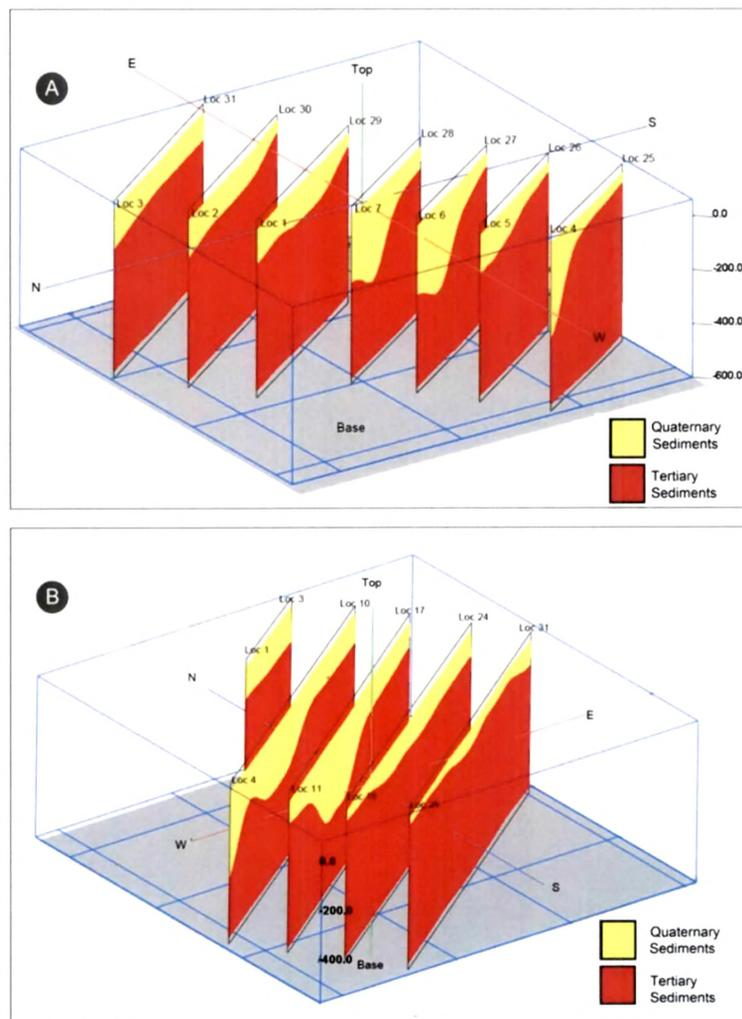
Figure 3-: Cross profiles showing the contact of unconsolidated soft sediment and consolidated bedrock variations of Quaternary sediments. (A) NW-SE profile and (B) NE-SW profiles.
