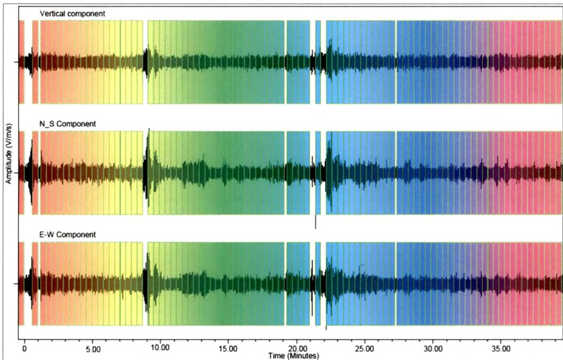
Figure 3:- An example of waveform recorded (Location 13) by Lennartz seismometer (5 s period) with City shark-II data acquisition system. X axis shows the time and Y axis shows the different components of amplitude viz. NS, EW and vertical.
