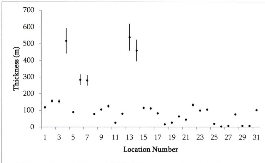
Figure 3-: Comparison between depths calculated using Ibs-von Seht and Wohlenberg (1999) and Parolai et al. (2002) relationships (Eqs. (2A) and (2B)). The circle indicates the average value whereas the length of the line suggests deviation from the average.
