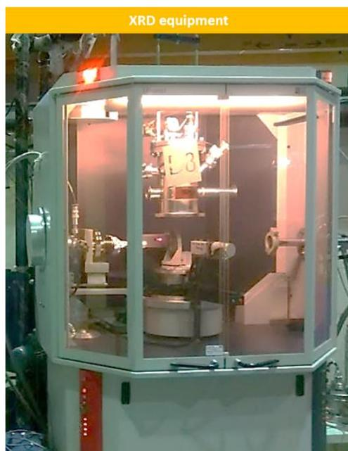
**Figure 2.4 Bruker D8-Advance diffractometer at IUAC, New Delhi**
