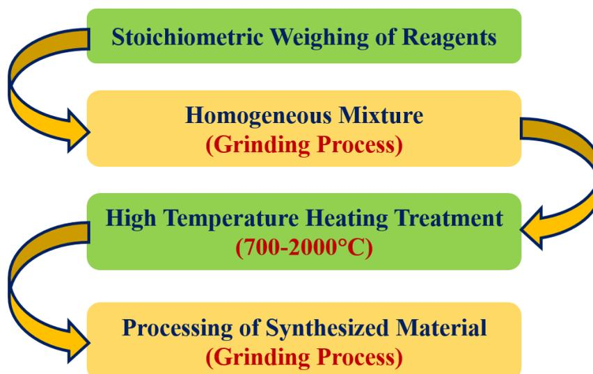
**Figure 2.3** Steps for conventional solid state reaction route.
