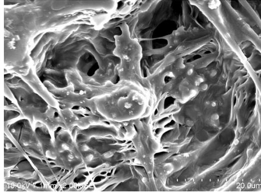
**Fig. 4.21(d)** SEM micrograph of PPS-17.5 sample irradiated at  $2 \times 10^{12}$  ions/cm<sup>2</sup> fluence
