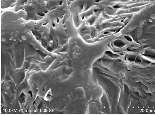
**Fig. 4.21(c)** SEM micrograph of PPS-17.5 sample irradiated at  $1 \times 10^{12}$  ions/cm<sup>2</sup> fluence.
