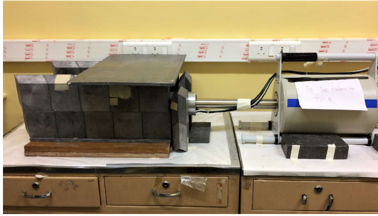
Figure 2.6: Pictorial view of typical source-detector counting setup at BARC-TIFR Pelletron facility
