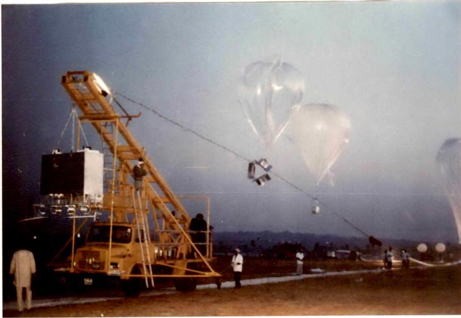
Figure 4.7: *Picture showing the payload assembly on the launch truck, alongwith the radar target, radiosonde etc. and the launch balloon, minutes before the launch.*
