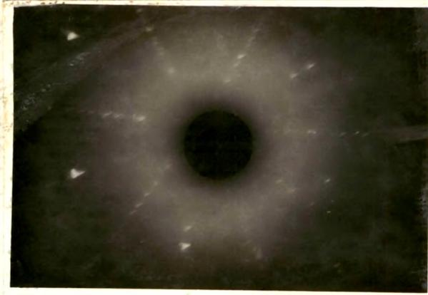
Figure - 5 : Laue back reflection pattern of the cleavage plane (0001) of  $\text{SnSe}_2$  single crystal.
