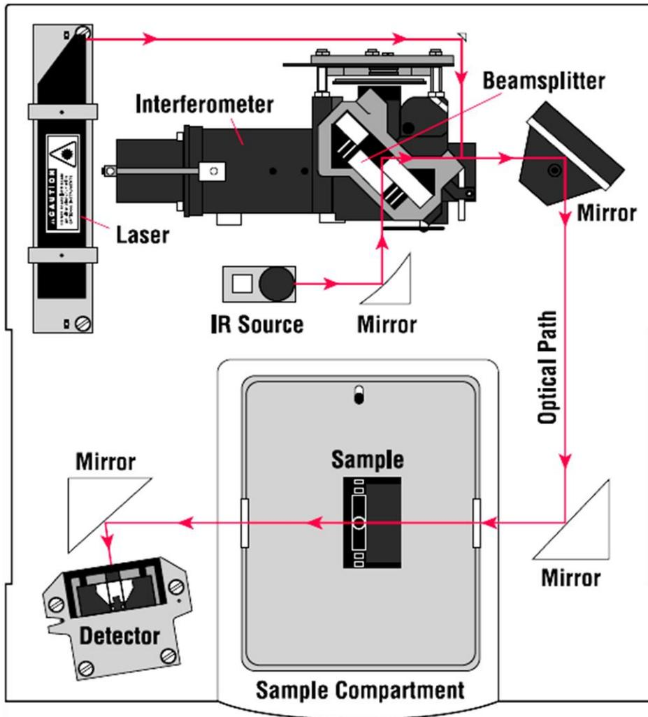
Fig. 3.7. Block Diagram of a typical FT-IR Spectrometer [3].
