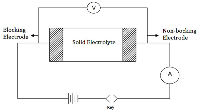
Fig. 3.12. Experimental arrangement of Wagner's polarization method for determining transport number.
