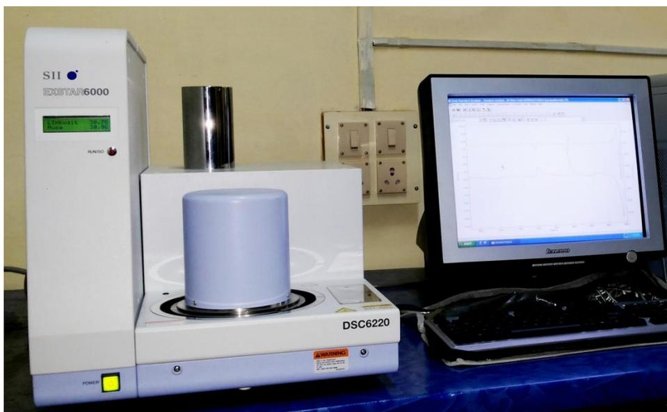
**Fig. 3.4. Image of the SII EXStar-6000 model DSC instrument.**
