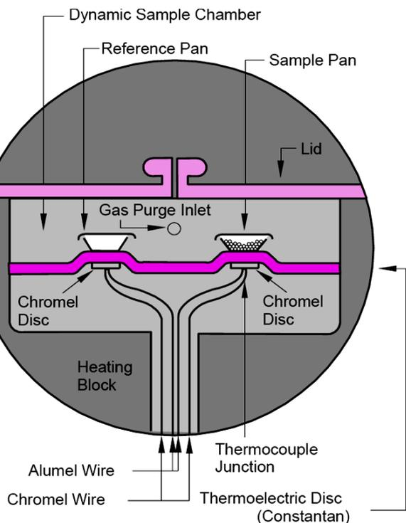
**Fig. 3.3. Schematic diagram of a basic heat flux DSC instrument.**
