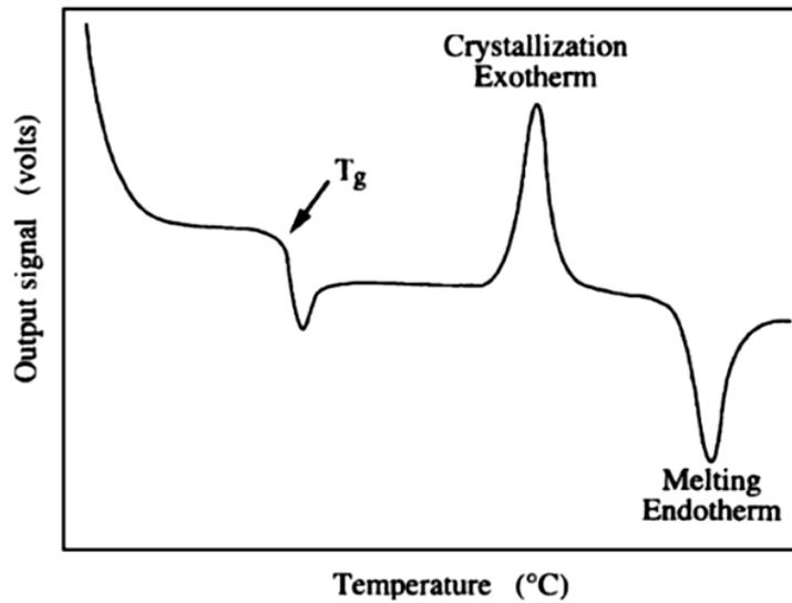
Fig. 3.5. A DSC curve exhibiting a change in specific heat at the glass transformation, an exothermic peak due to crystallization of the glass, and an endotherm due to melting of the crystals formed at the exotherm. (Reproduced from Ref. [1] )
