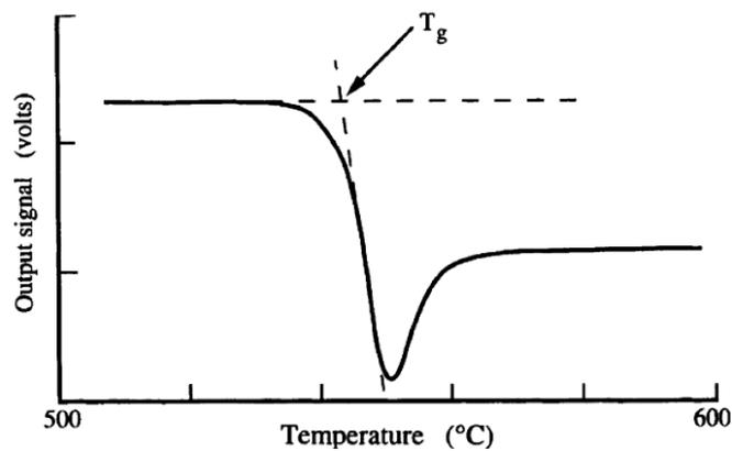
Fig. 3.6. An example of the determination of glass transition temperature,  $T_g$  from a DSC curve. (Reproduced from Ref. [1]).
