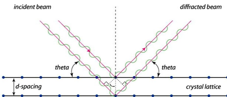
**Fig. 3.1. Schematic representation of diffraction of X-rays by a crystal.**
