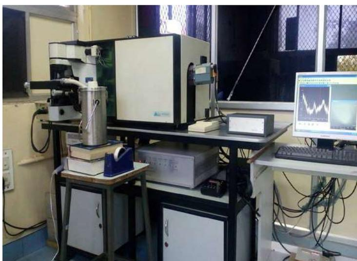
**Fig. 2.11:** Instrument set-up of Raman Spectroscopy.
