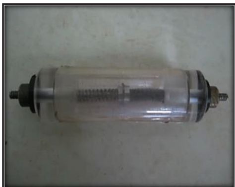
Fig. 3.21 (a) ' \text{Ag}^+ primary polymer battery' assembly
