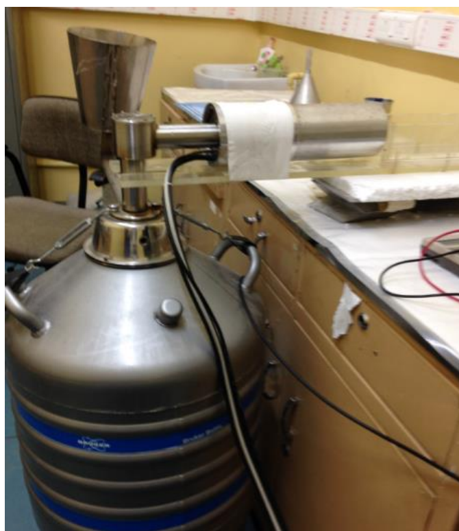
FIG 4.1(c) Gamma spectroscopy system for activity measurement
