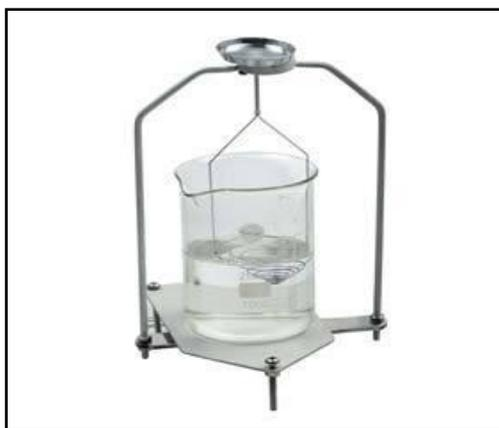
Fig. 3.5 Assembly of weighing pan immersed in methanol
