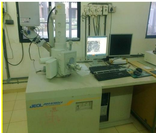
**Fig. 3.6** Experimental setup of Scanning Electron Microscope interfaced with computer
