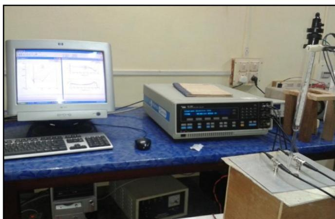
**Fig. 3.13 Experimental setup of Solartron Impedance Analyser interfaced with computer.**
