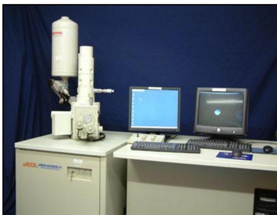
**Fig. 3.10** Experimental setup of EDS interfaced with SEM instrument and a controlling computer
