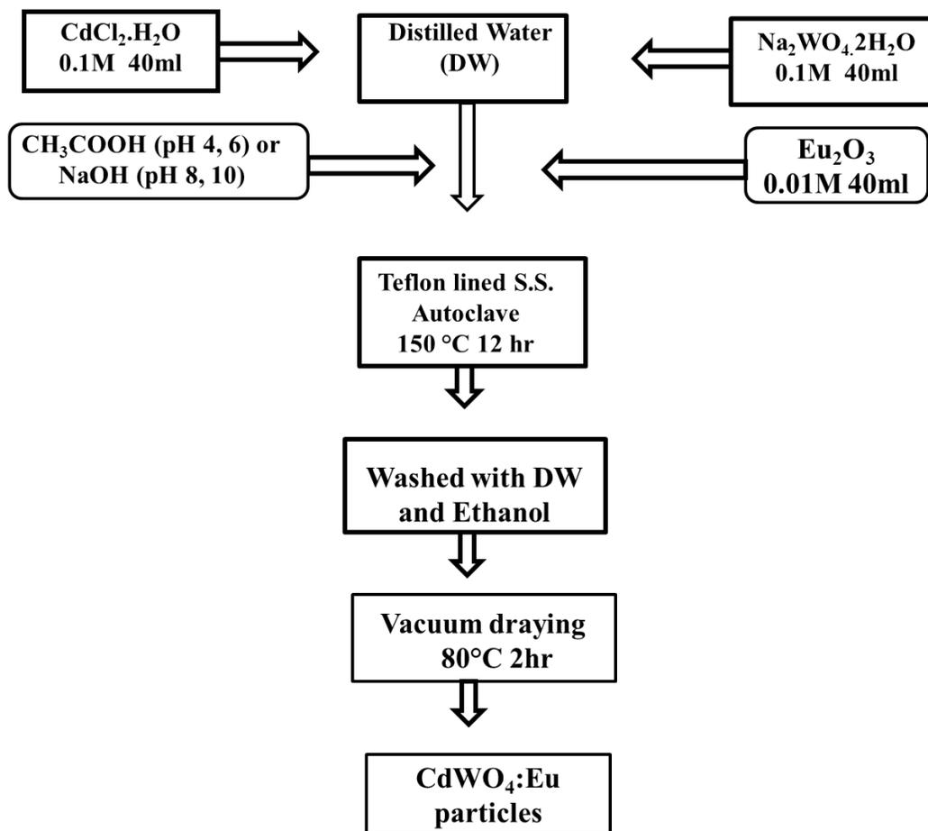
**Figure 6.1** Flow chart of Europium doped CdWO<sub>4</sub> synthesized at pH (4, 6, 8, 10) .
