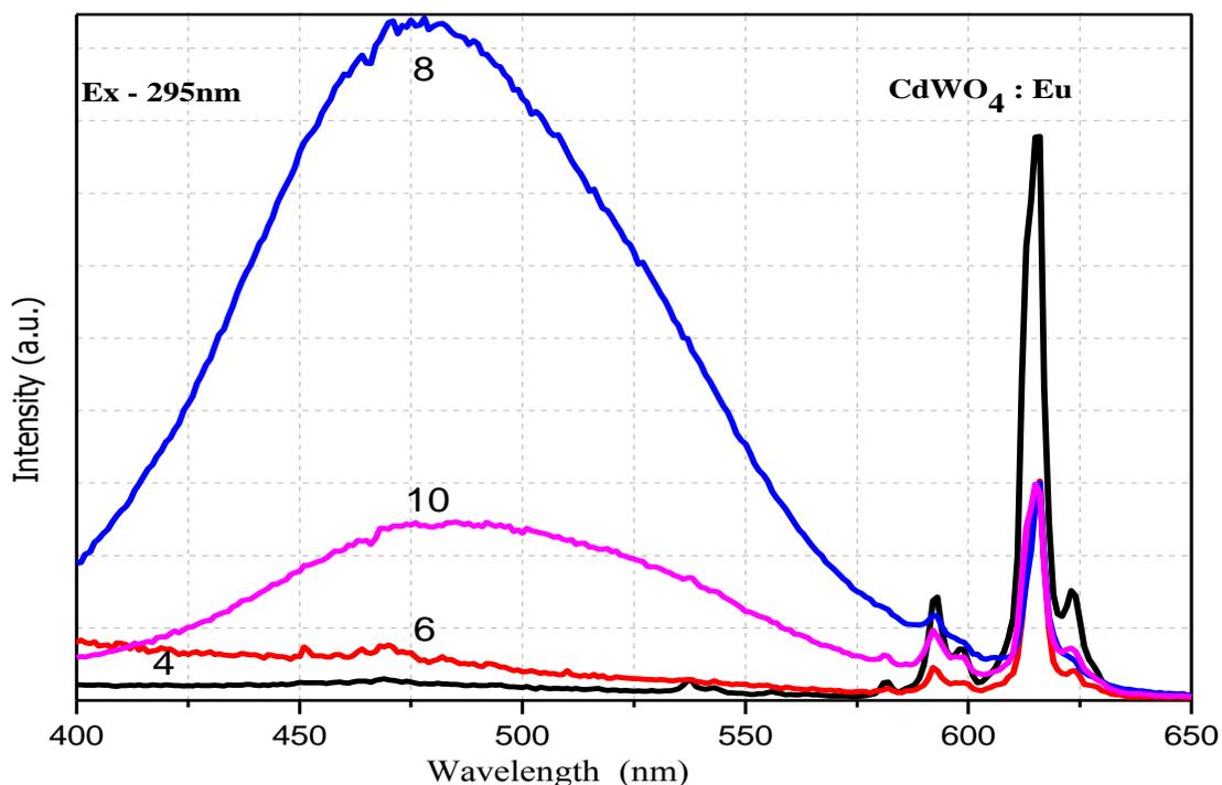
**Figure 6.5** Emission spectra of Europium doped  $\text{CdWO}_4$  synthesized at pH (4, 6, 8, 10).
