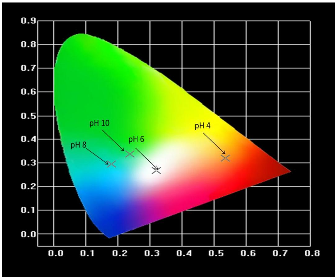
**Figure 6.6** CIE chromaticity diagram with points indicating coordinates for Europium doped CdWO<sub>4</sub> synthesized at different pH (4, 6, 8,10) recorded with 295 nm excitation wavelength.
