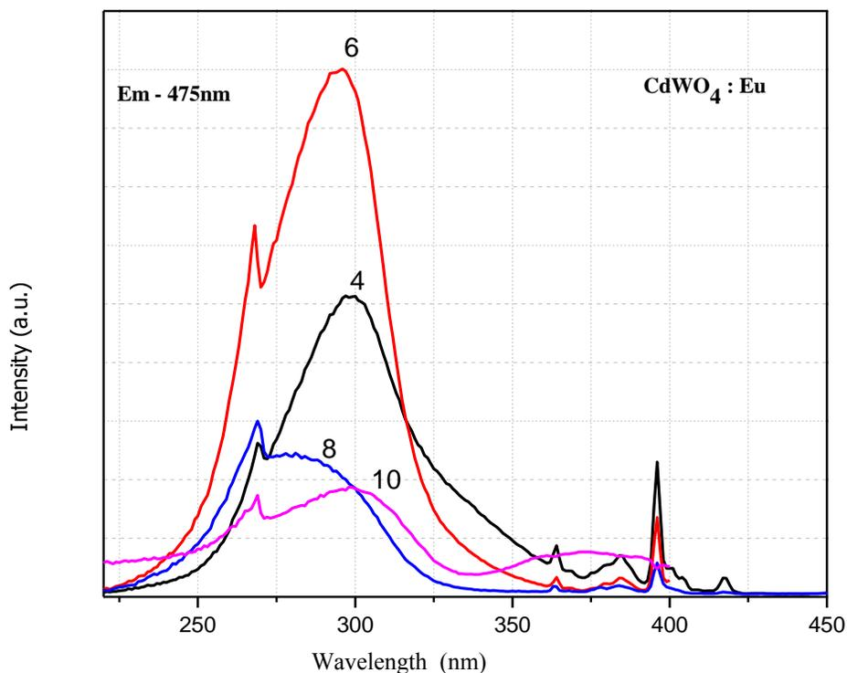
**Figure 6.4** Excitation spectra of Europium doped  $\text{CdWO}_4$  synthesized at pH(4, 6, 8, 10).
