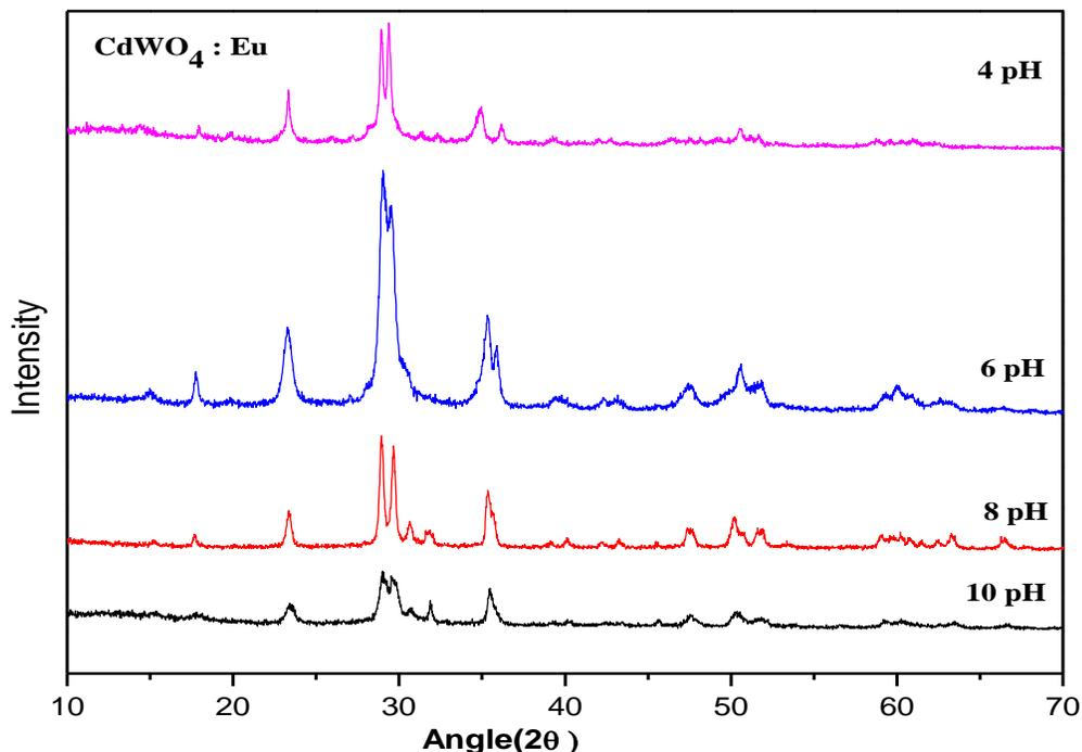
**Figure 6.2** XRD patterns of Europium doped  $\text{CdWO}_4$  synthesized at pH (4, 6, 8, 10)
