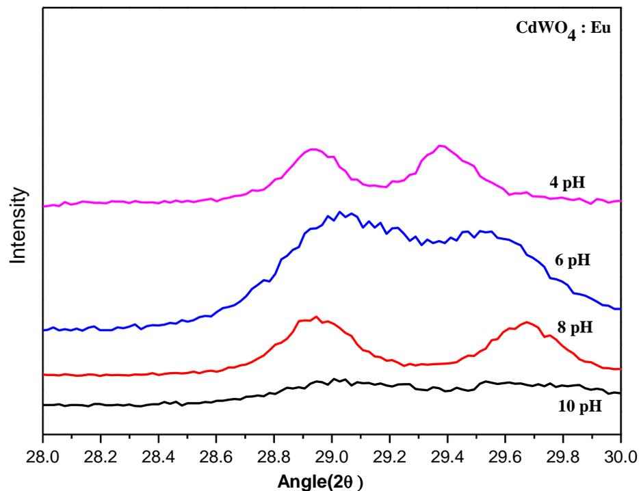
**Figure 6.3** Shift of reflection peak of Europium doped  $\text{CdWO}_4$  synthesized at pH (4, 6, 8, 10).
