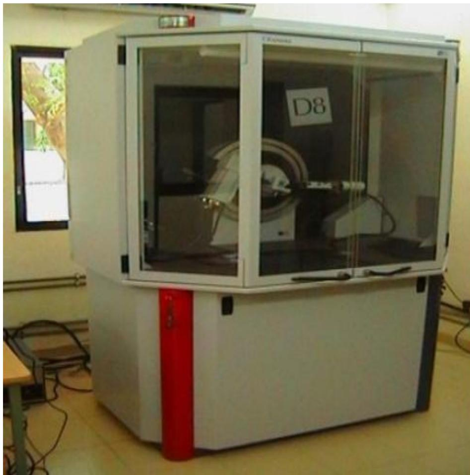
**Figure 3.5** XRD instrument at ERDA, Vadodara.
