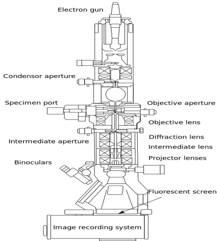
**Figure 3.9** Layout of optical components in a basic TEM [25]
