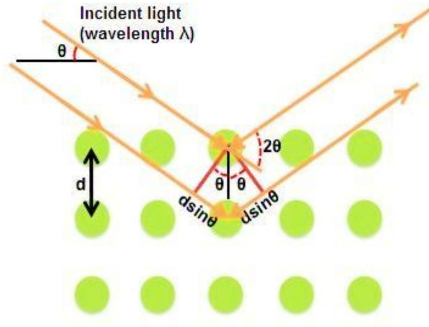
**Figure 3.2** Schematic representation of x-ray diffraction pattern.
