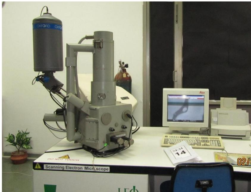
**Fig. 6 Scanning Electron Microscope and EDAX System Setup**
