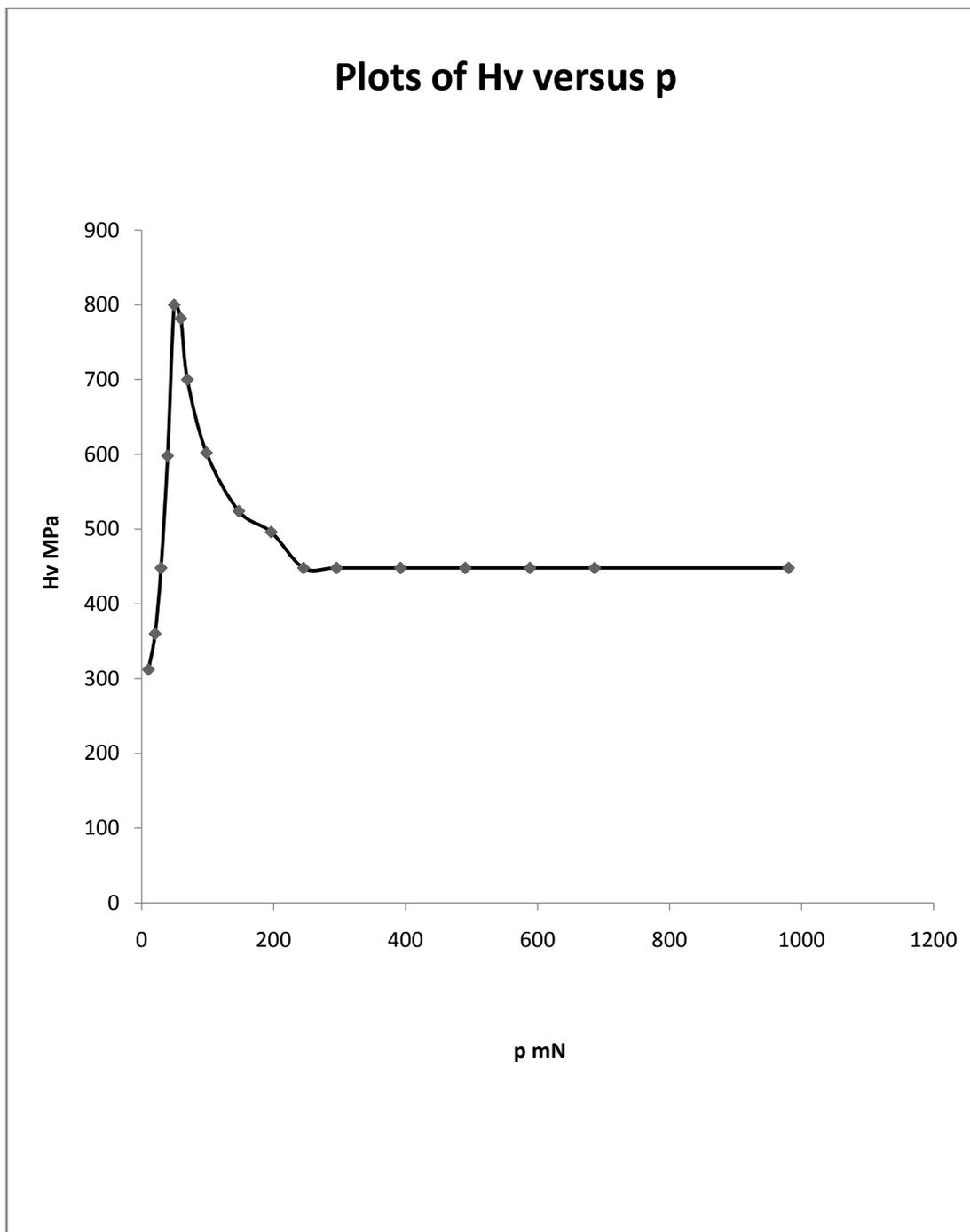
Figure -2 Plots of  $H_v$  versus  $p$  for  $\text{Bi}_2\text{Te}_3$  crystals
