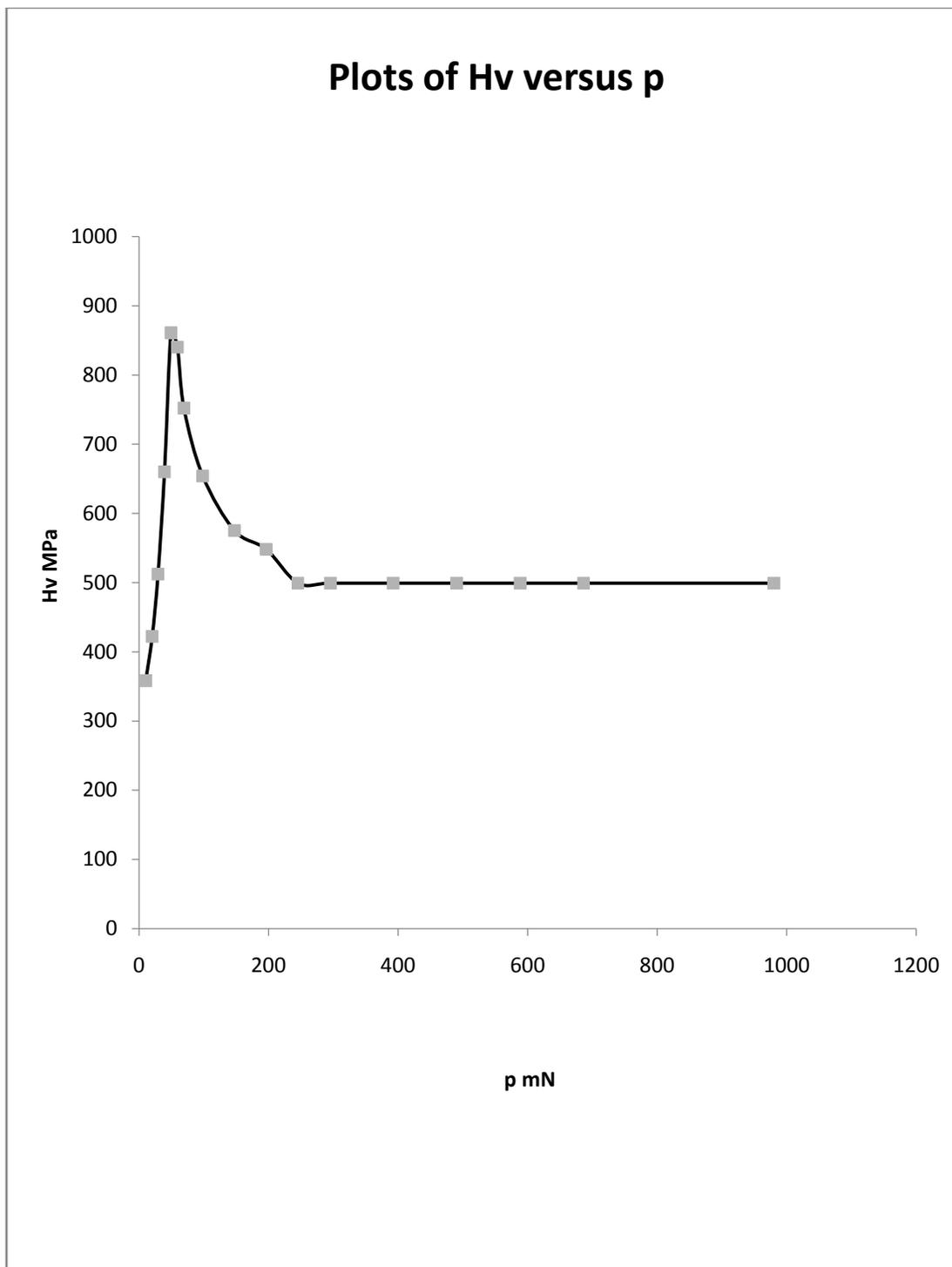
Figure -3 Plots of  $H_v$  versus  $p$  for  $\text{Bi}_{1.95}\text{Sb}_{0.05}\text{Te}_3$  crystal
