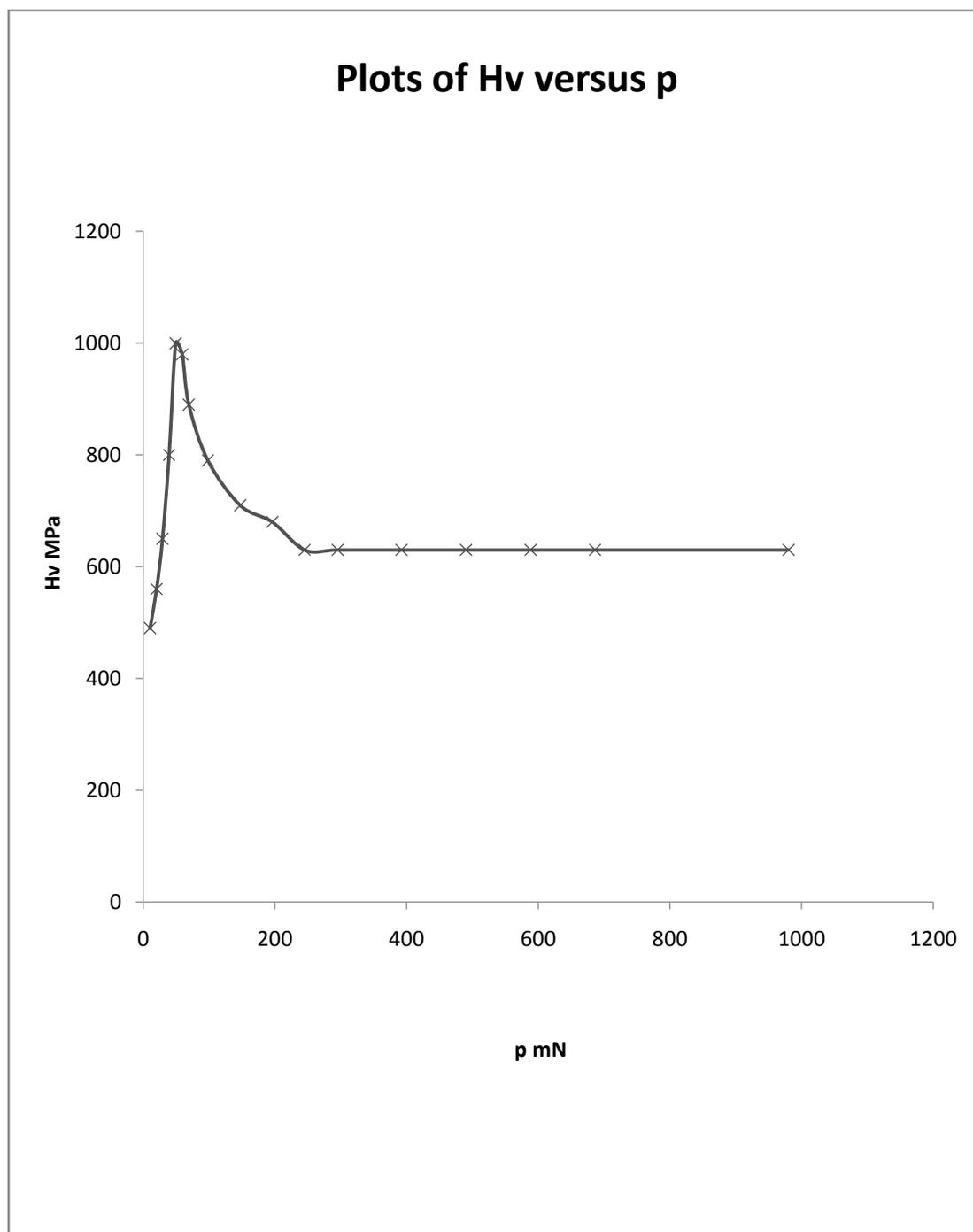
Figure –5 Plots of  $H_v$  versus  $p$  for  $\text{Bi}_{1.80}\text{Sb}_{0.2}\text{Te}_3$  crystal
