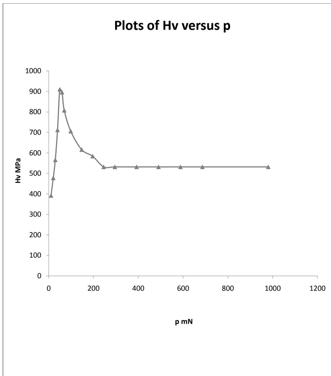
Figure –4 Plots of  $H_v$  versus  $p$  for  $\text{Bi}_{1.90}\text{Sb}_{0.1}\text{Te}_3$  crystal
