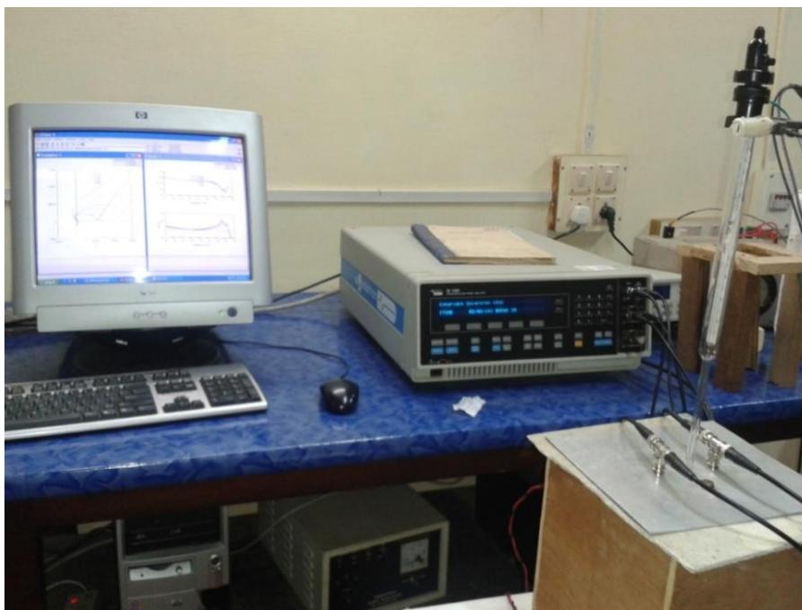
**Fig.3.23** Image of setup of impedance measurement (Impedance analyzer interfaced with computer).
