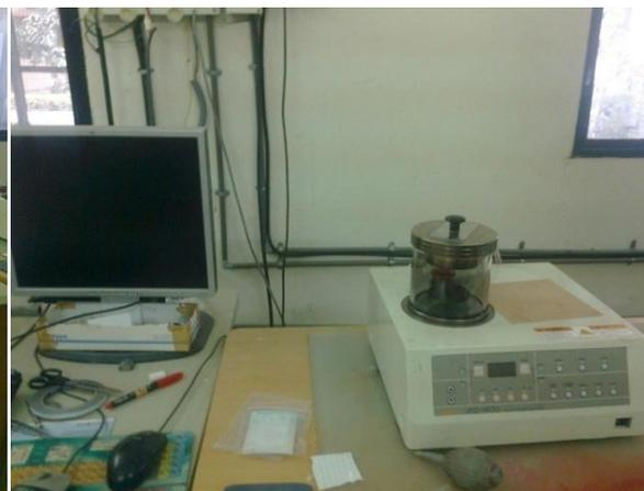
**Fig. 3.13** Image of the gold/palladium source coating unit for SEM studies.
