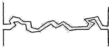
Figure 1.2 : Mechanism of adhesion : Mechanical interlocking
