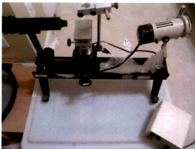
Figure 2.4: Contact angle goniometer (NRL C.A. Goniometer, Model 100-00-230)
