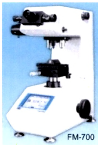
Figure 2.7: Vicker's Microhardness Indenter Future Tech. (FM-700)
