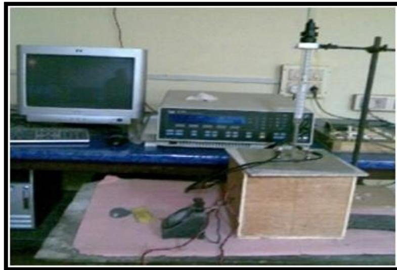
Fig. 3.8 AC Conductivity measurement setup
