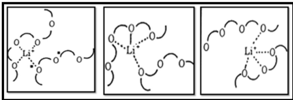
Fig. 1.2 Schematic diagram of fast ion conduction [12]
