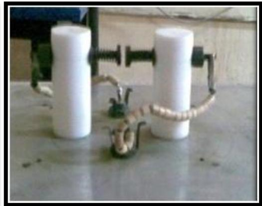
Fig. 3.7 Sample holder for the conductivity measurements.
