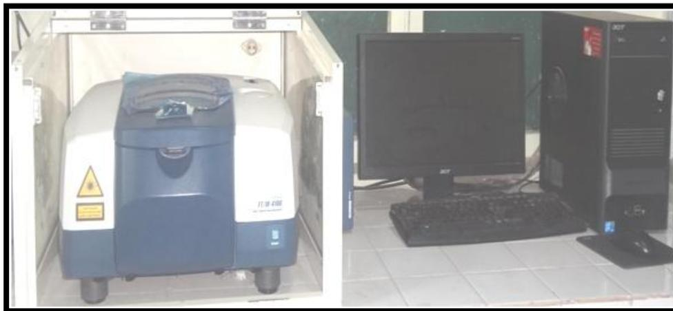
**Fig. 3.1** Image of FTIR instrument.
