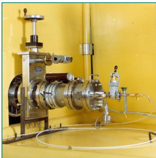
**Fig 3.24:** SNICS source using in FOTIA facility for beam ion extraction.
