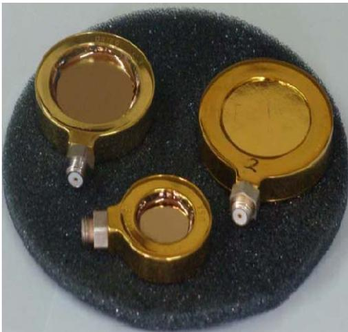
**Fig 3.6:** Typical solid state detector used in nuclear physics experiments
