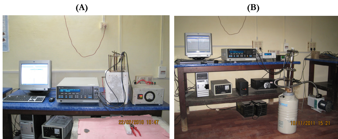
Figure 3.12: (A) The impedance spectroscopy setup for high temperature measurement. (B) The impedance spectroscopy setup for low temperature measurement.
