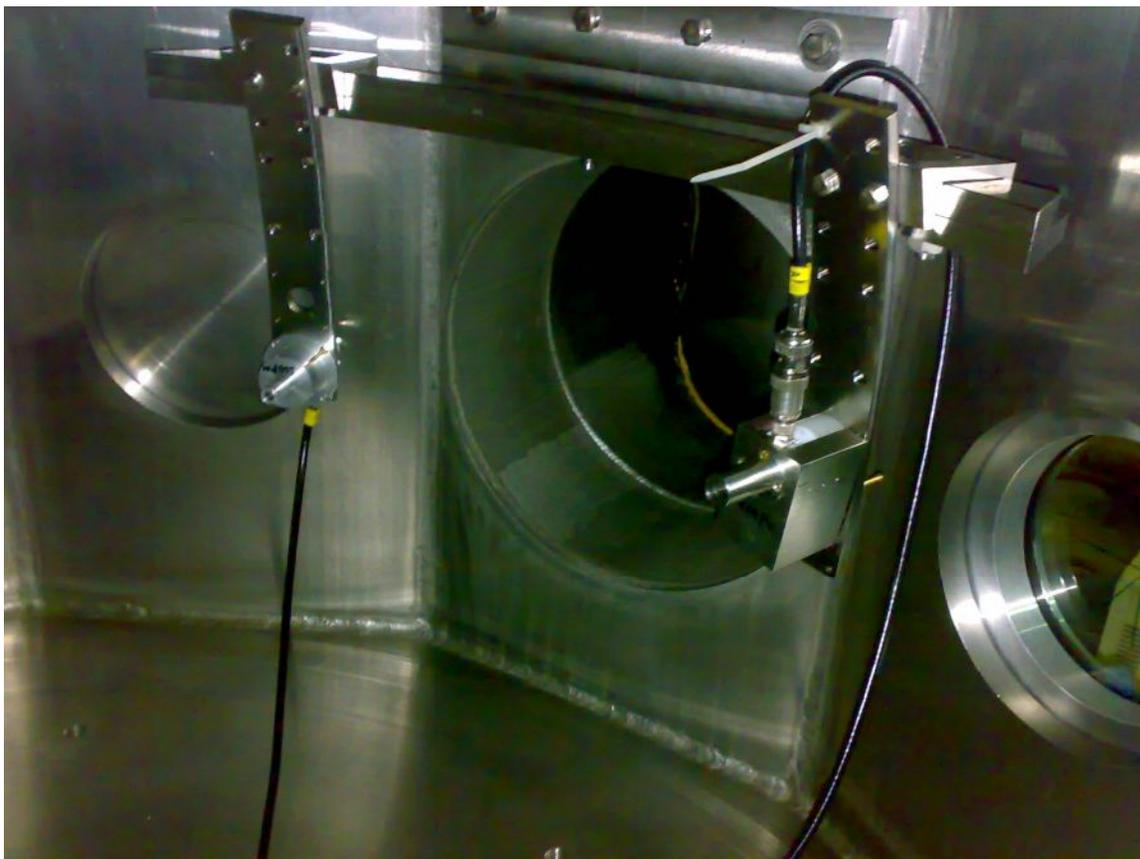
**Figure 3.3 (b) Two monitor detectors for absolute normalization were kept hanging (fixed) in the scattering chamber at  $\pm 20^\circ$ .**
