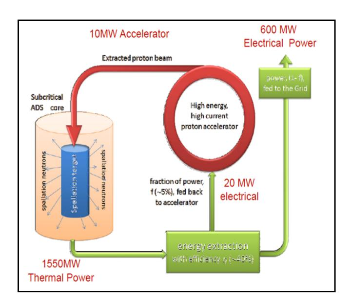
Fig. 2.2 A Schematic diagram of ADS
