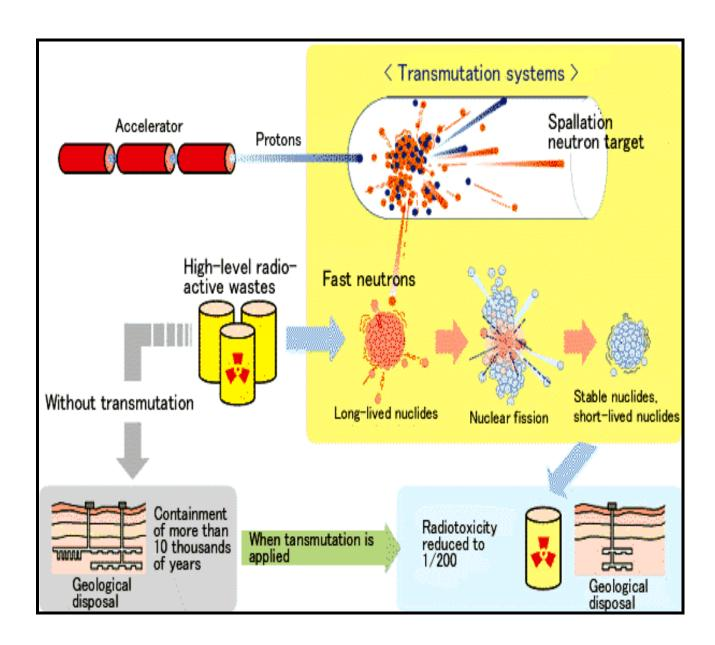
Fig. 2.3 A Schematic diagram of ADS for transmutations
