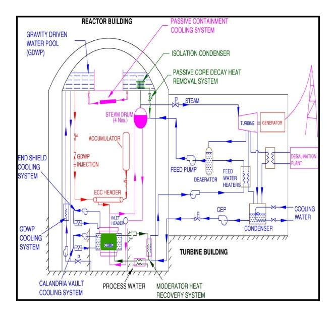
Fig. 2.1 A schematic arrangement of the AHWR [1]
