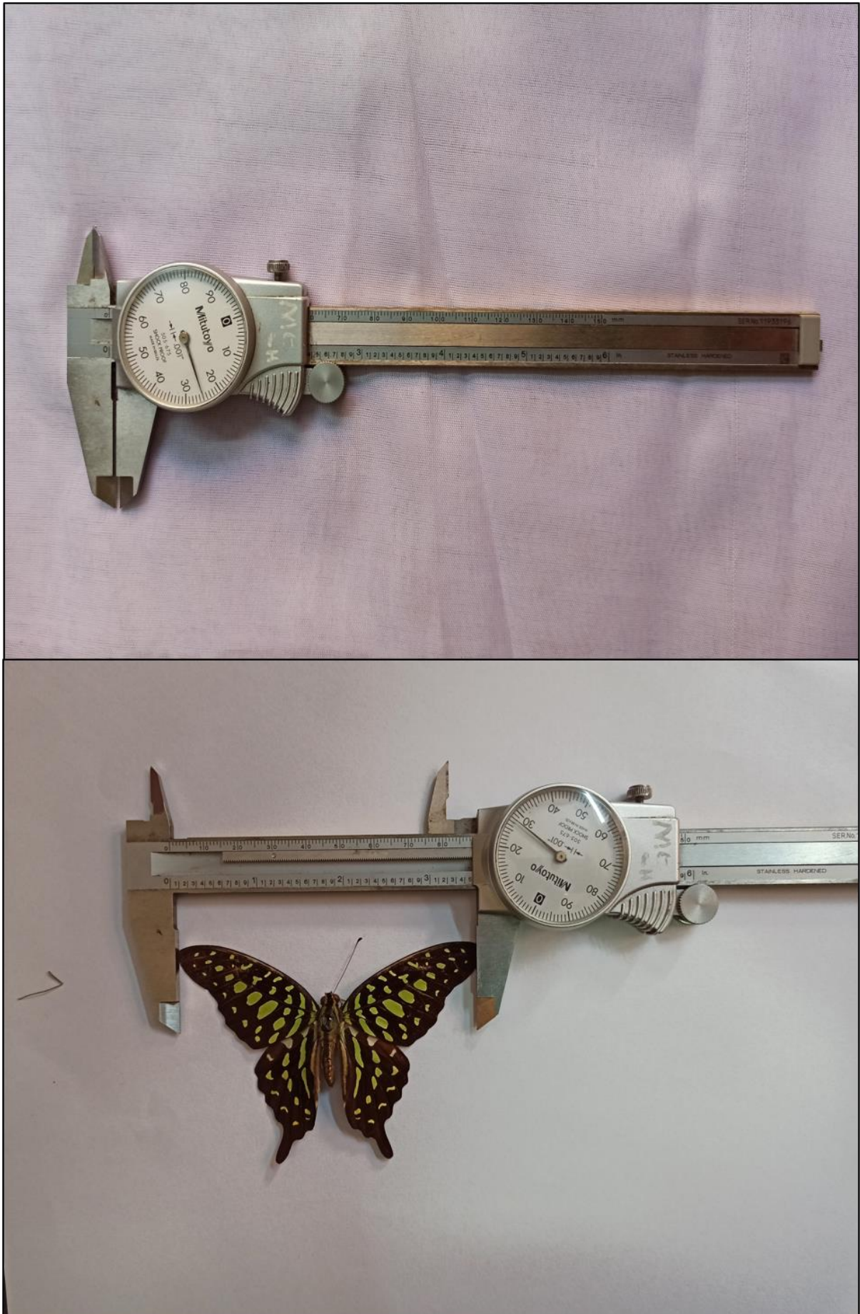
Figure 13: Dial Calliper used in morphometry studies
