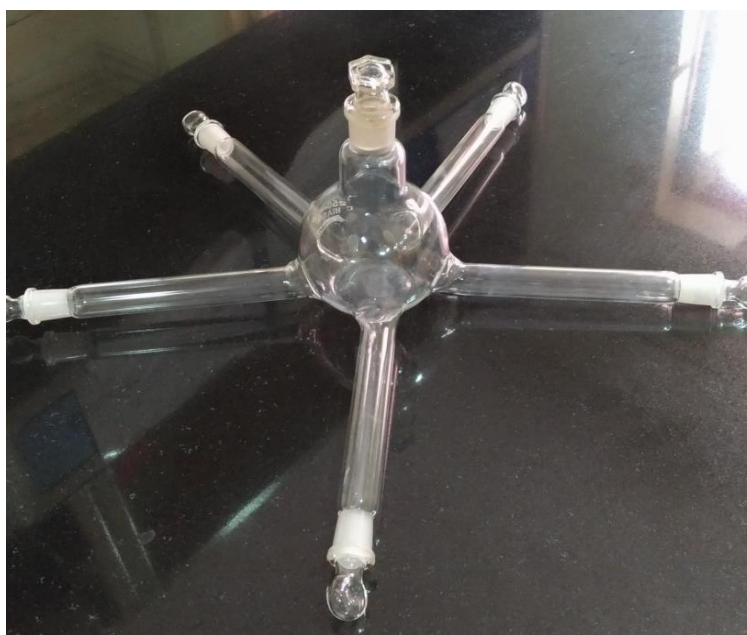
Figure 4: Multi arm olfactometer for behavioural bioassay in response to EOs Technical details of the olfactometer are as follows: middle glass chamber: 7 cm in diameter; arms: 1.5 cm in diameter & 14.5 cm in length. In the bioassay, filter papers were cut into two equal halves (Figure 4). Paper halves measuring about 3.5 cm were then treated with the different concentrations of EOs and
