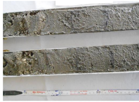
Core pipe showing fine sand with silt horizons.
