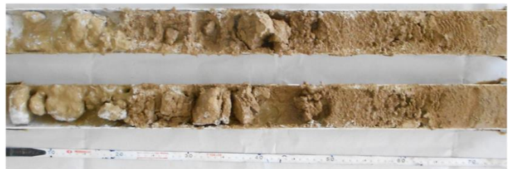
The lower fluvial sequence showing the semi-compacted nature of the sediments and palaeosol.
