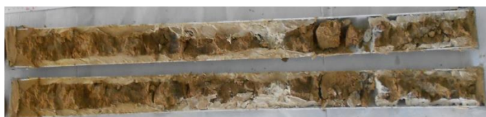
Sand and silt as well as red palaeosol horizons observed within RMD core
