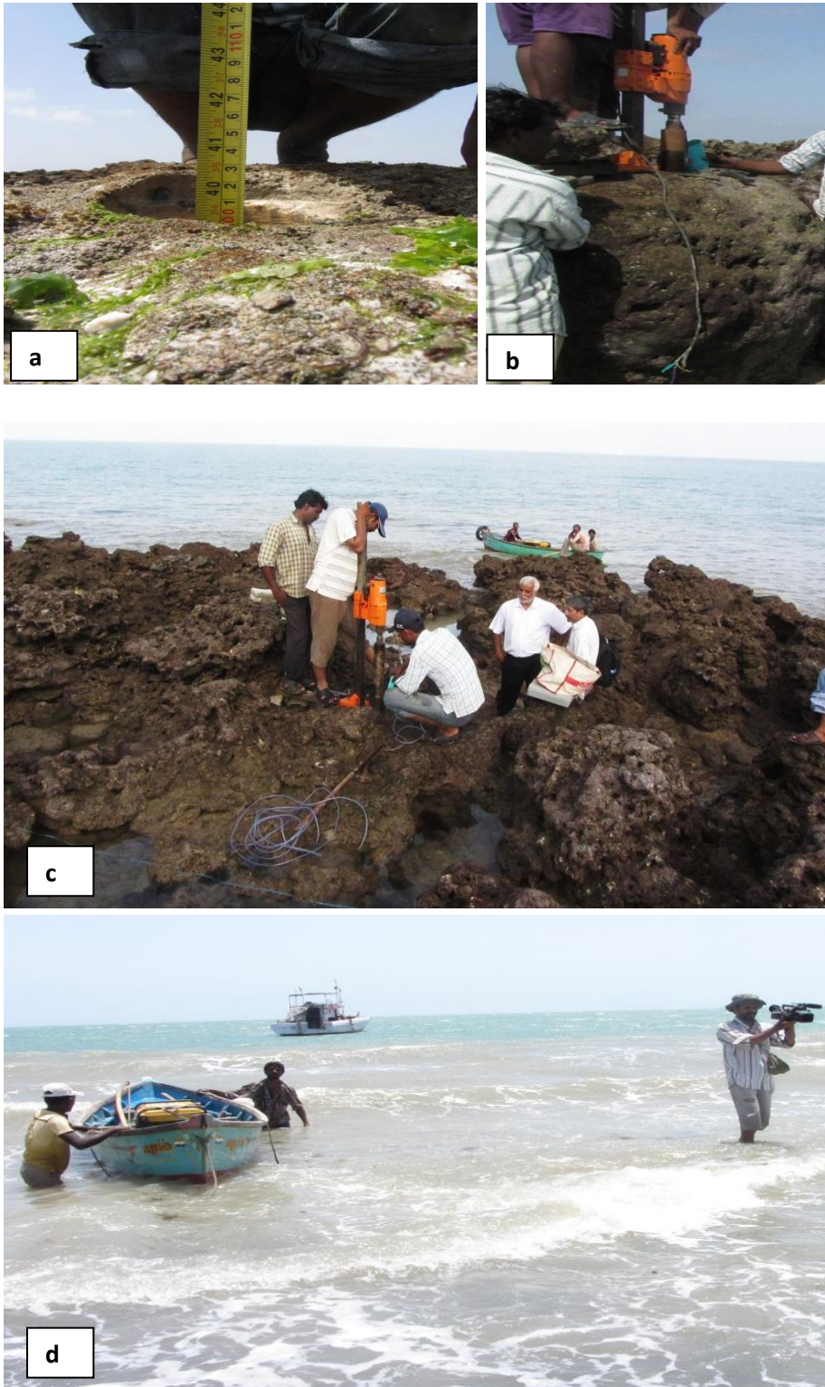
Plate:4.2- Field Procedures: a-measuring the drilled hole; b-partially drilled core; c-Drilling going on at very uneven and difficult reef surface; d-Field difficulty- Boatmen partially in water, holding the boat against high tide waters of the GoK.
