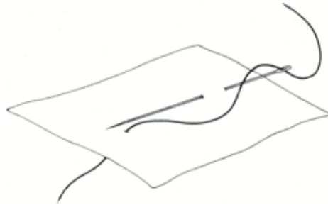
Figure 2.5a: A long stitch is made first. It starts and ends in an entire area of the textile and crosses the weak or damaged area. Lining fabric and degraded area of textile not shown.
