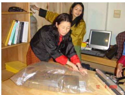
Plate 2.24: Purging the bag with nitrogen
