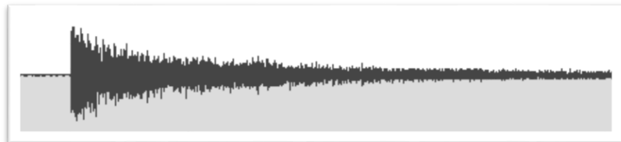
Fig. 4.3 Sound Envelope of Striking a Cymbal with a Stick
