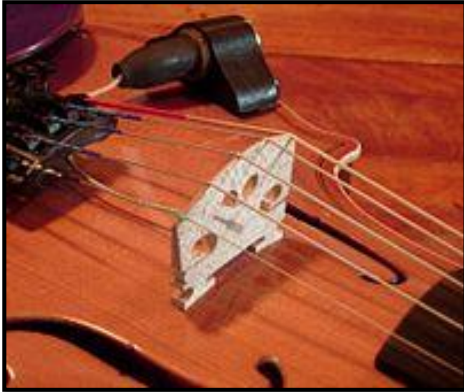
Fig 5.10 Piezoelectric Violin Bridge Pickup
